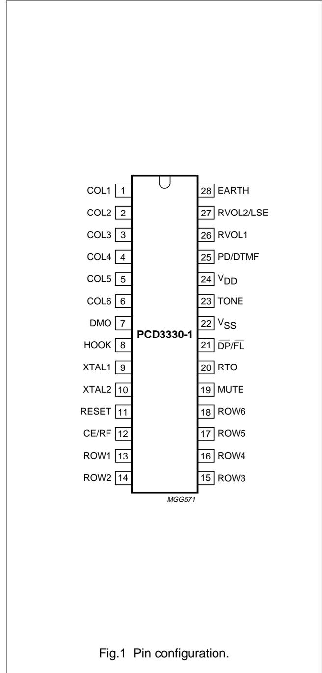
Fig.1 Pin configuration.
