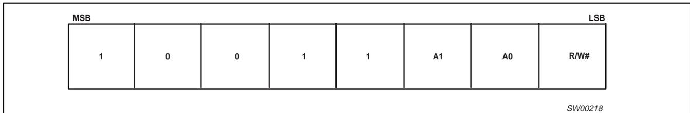
Figure 1. I<sup>2</sup>C Address Byte
