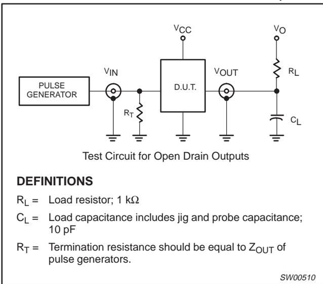
Test Circuit for Open Drain Outputs
