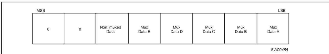
Figure 2. I<sup>2</sup>C Data Byte
