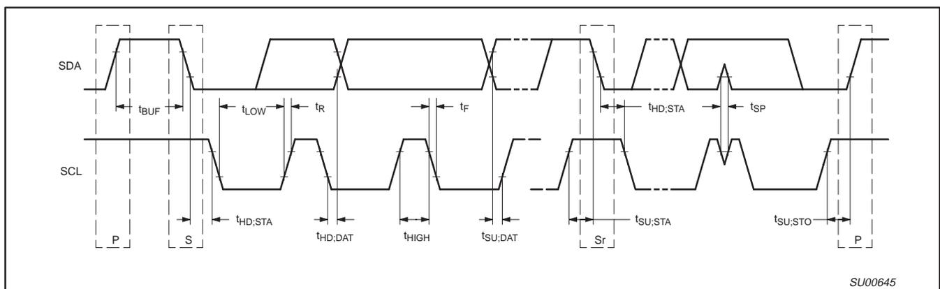
Figure 13. Definition of timing on the I<sup>2</sup>C-bus
