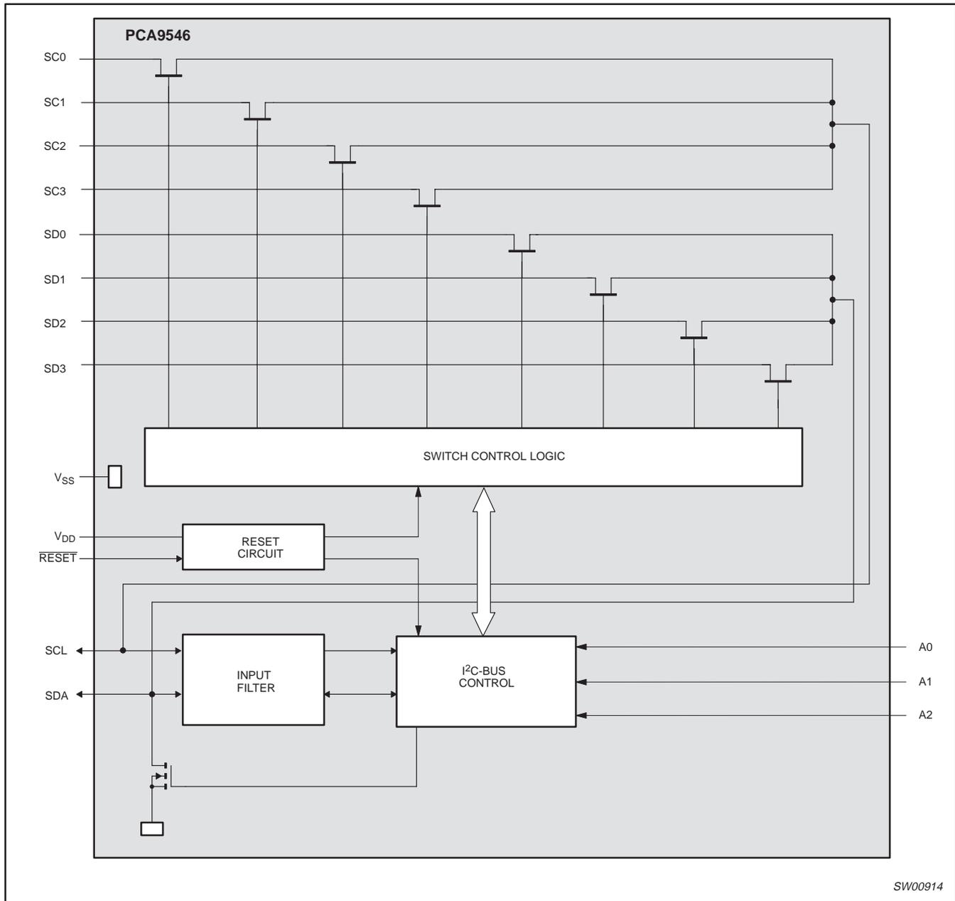
Figure 2. Block diagram
