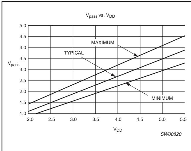
Figure 5. V<sub>pass</sub> voltage vs. V<sub>DD</sub>
