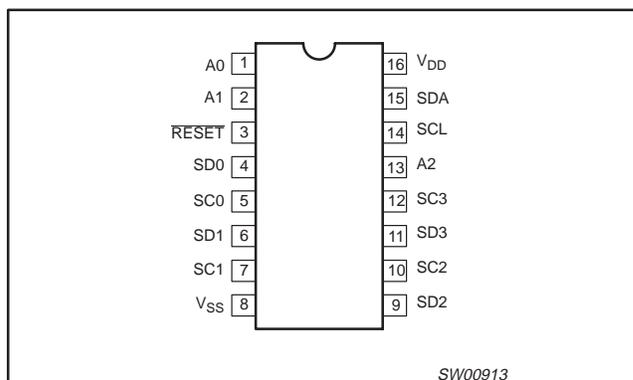
Figure 1. Pin configuration
