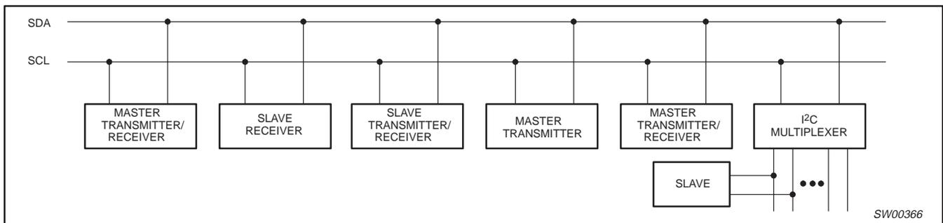
Figure 8. System configuration
