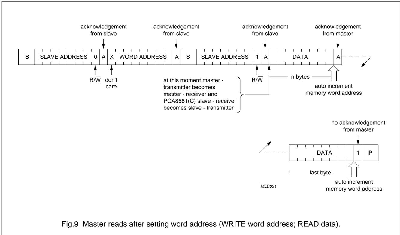
Fig.9 Master reads after setting word address (WRITE word address; READ data).
