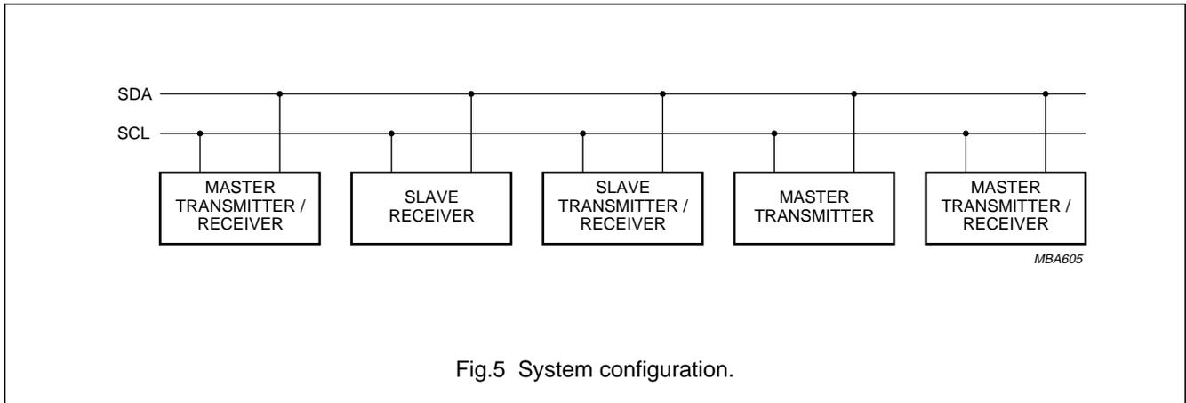
Fig.5 System configuration.
