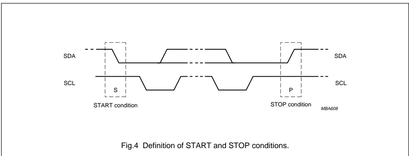
Fig.4 Definition of START and STOP conditions.
