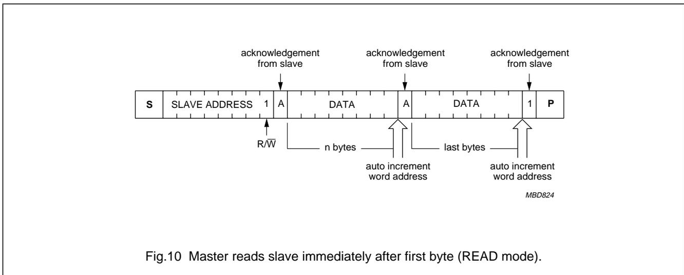
Fig.10 Master reads slave immediately after first byte (READ mode).
