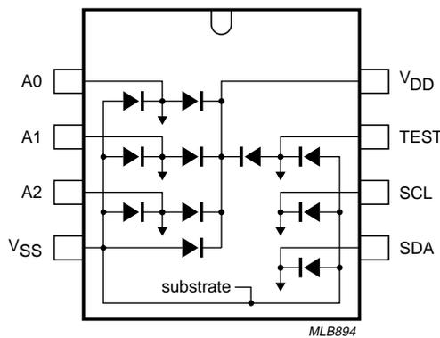
There is no connection between SCL and V<sub>DD</sub>, and SDA and V<sub>DD</sub>; this allows powering down the device without affecting I<sup>2</sup>C-bus operation.
