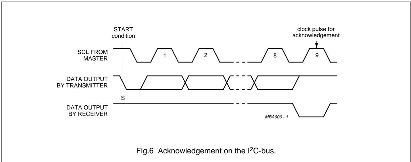
Fig.6 Acknowledgement on the I<sup>2</sup>C-bus.
