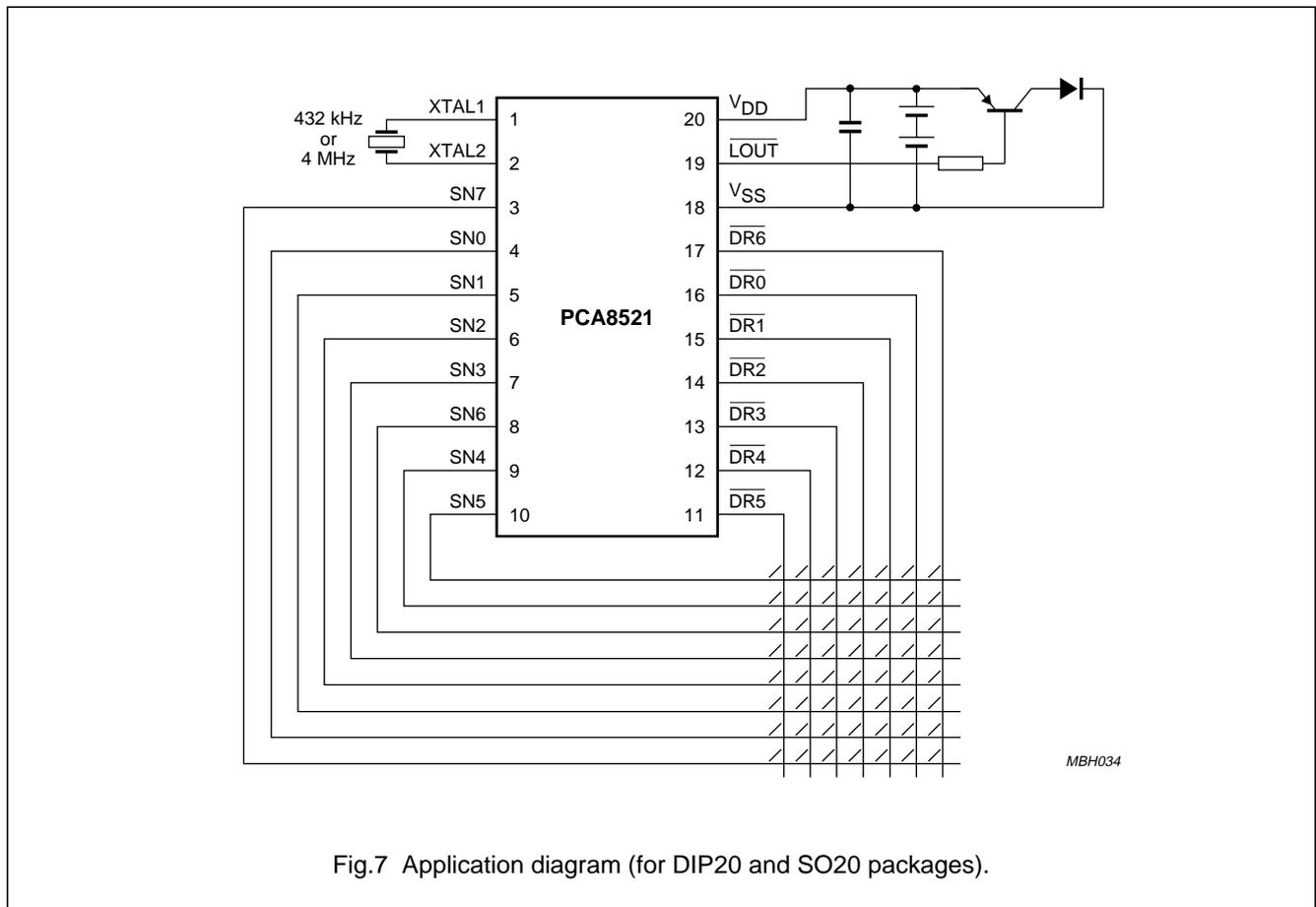
Fig.7 Application diagram (for DIP20 and SO20 packages).
