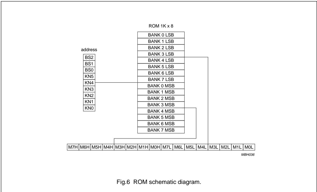
Fig.6 ROM schematic diagram.
