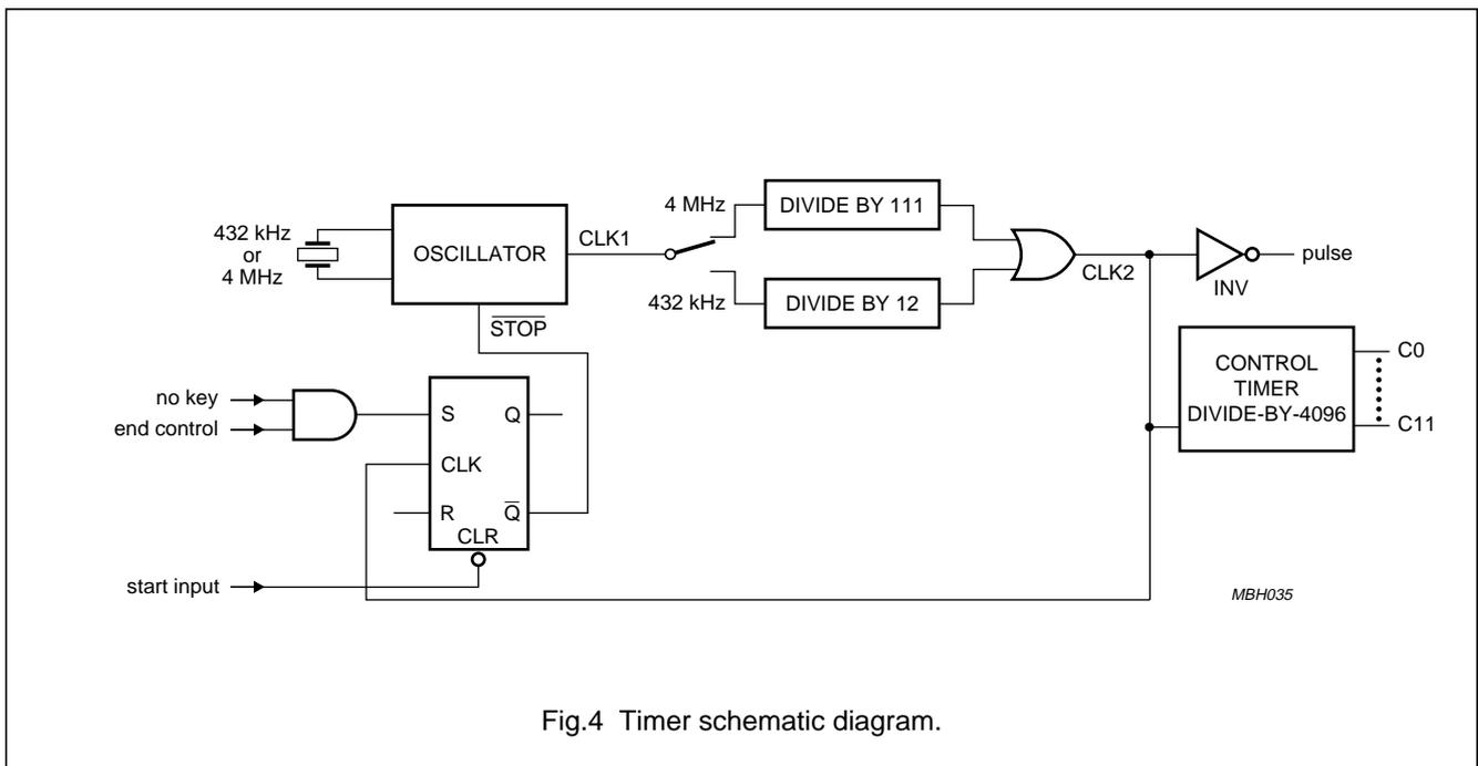
Fig.4 Timer schematic diagram.
