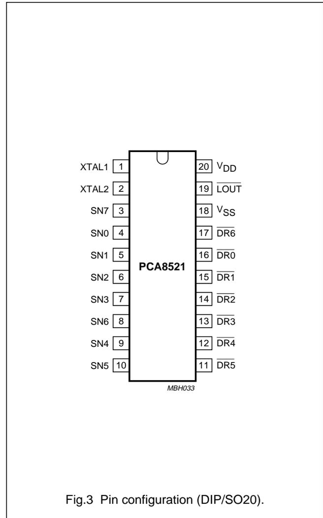
Fig.3 Pin configuration (DIP/SO20).
