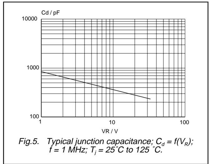
Fig.5. Typical junction capacitance;  $C_d = f(V_R)$ ;  $f = 1\text{ MHz}$ ;  $T_j = 25\text{ C to } 125\text{ C}$ .
