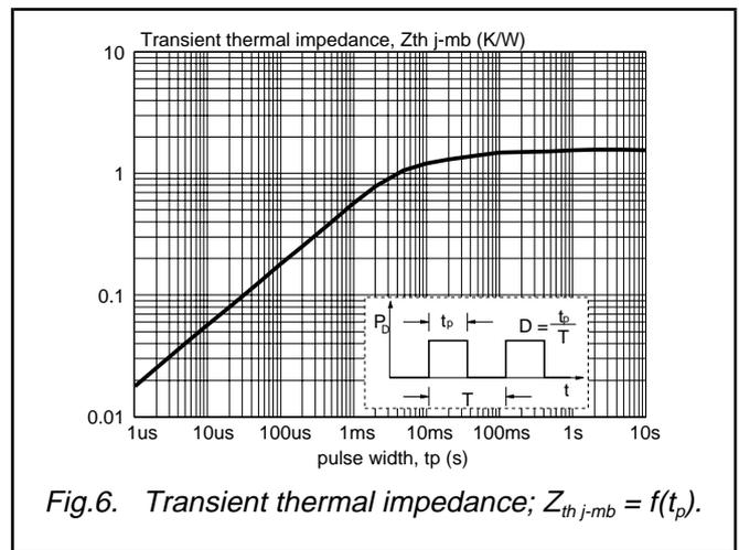
Fig.6. Transient thermal impedance;  $Z_{th\ j-mb} = f(t_p)$ .
