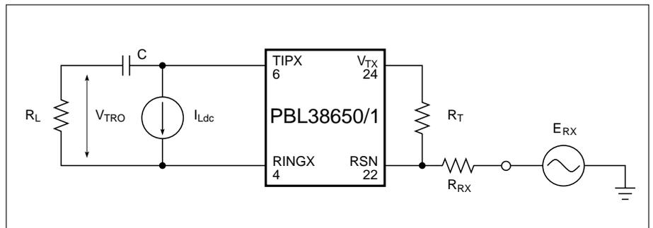
Figure 3. Longitudinal to metallic (B<sub>LME</sub>) and Longitudinal to four-wire (B<sub>LFE</sub>) balance
