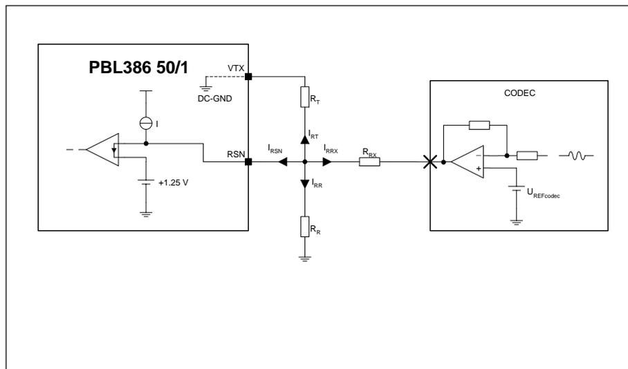
Figure 14. CODEC receive interface.
