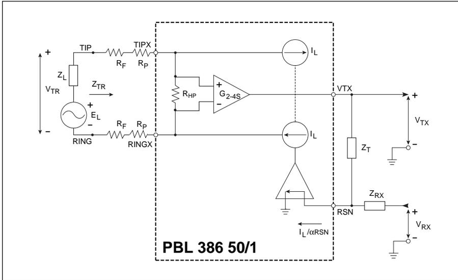
Figure 10. Simplified ac transmission circuit.
