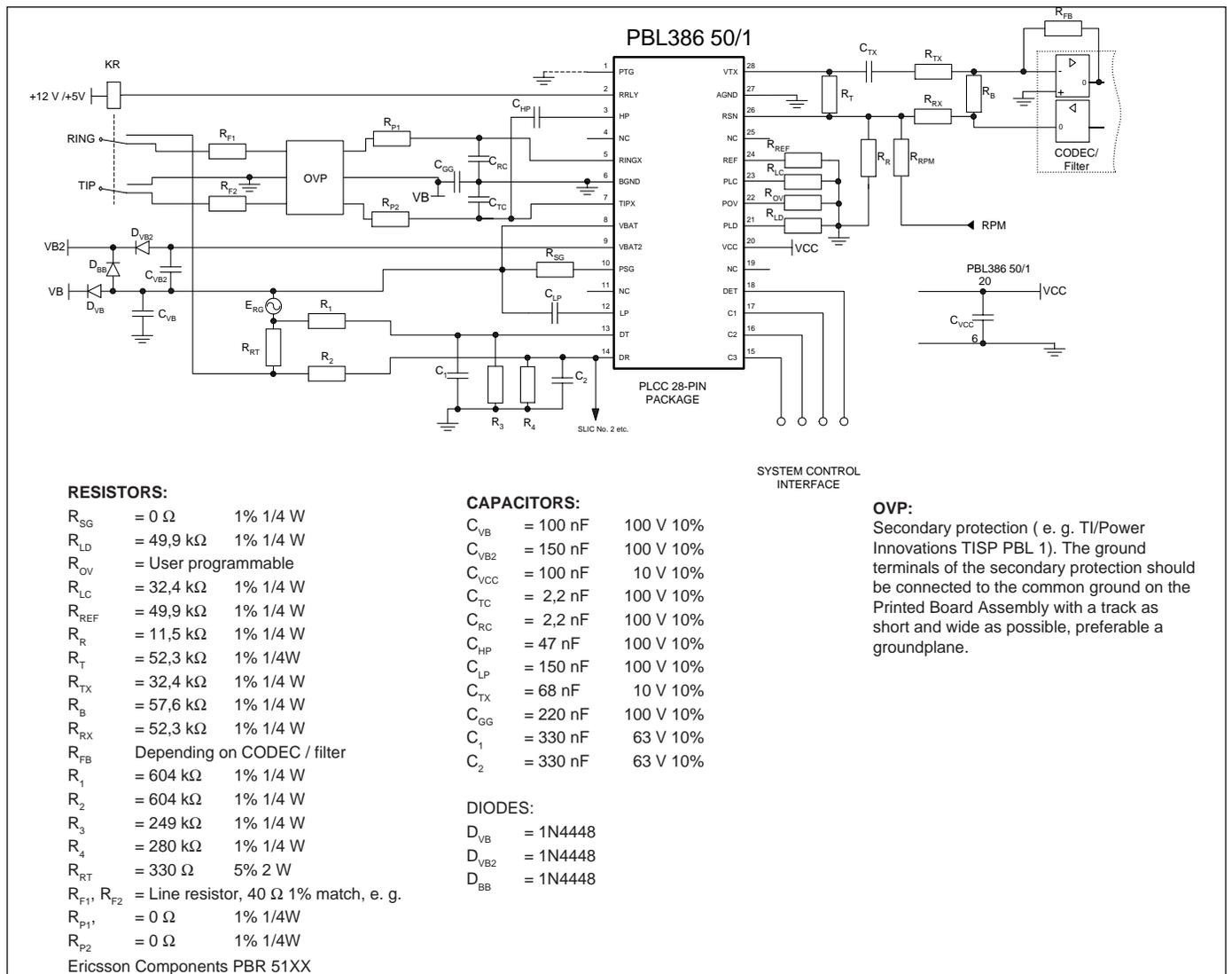
Figure 12. Single-channel subscriber line interface with PBL 386 50/1 and combination CODEC/filter.
