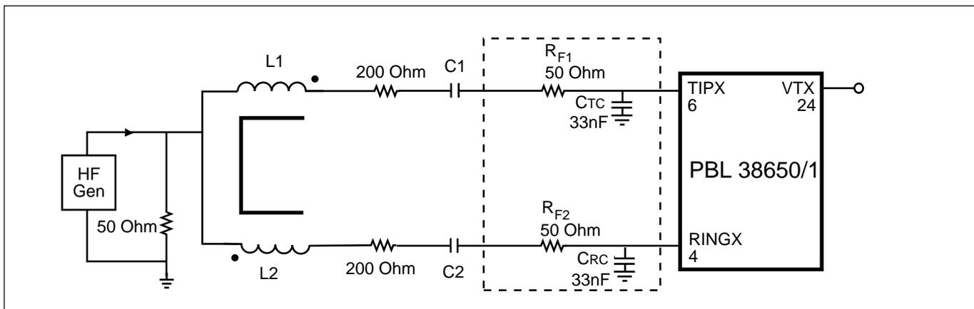
Figure 8. RFI Test Circuit.
