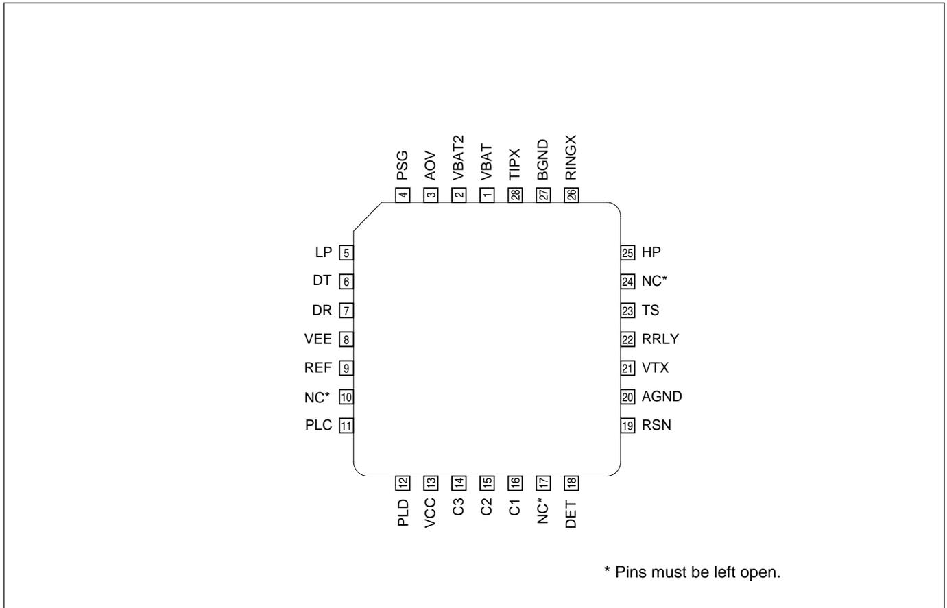
Figure 8. Pin configuration, 28 pin PLCC package, top view.
