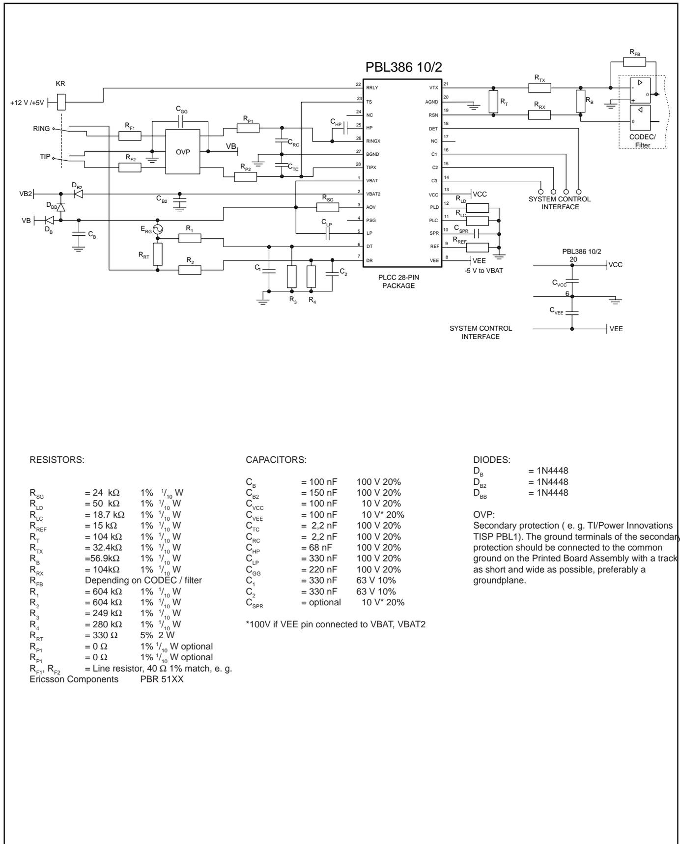
Figure 12. Single-channel subscriber line interface with PBL 386 10/2 and combination CODEC/filter
