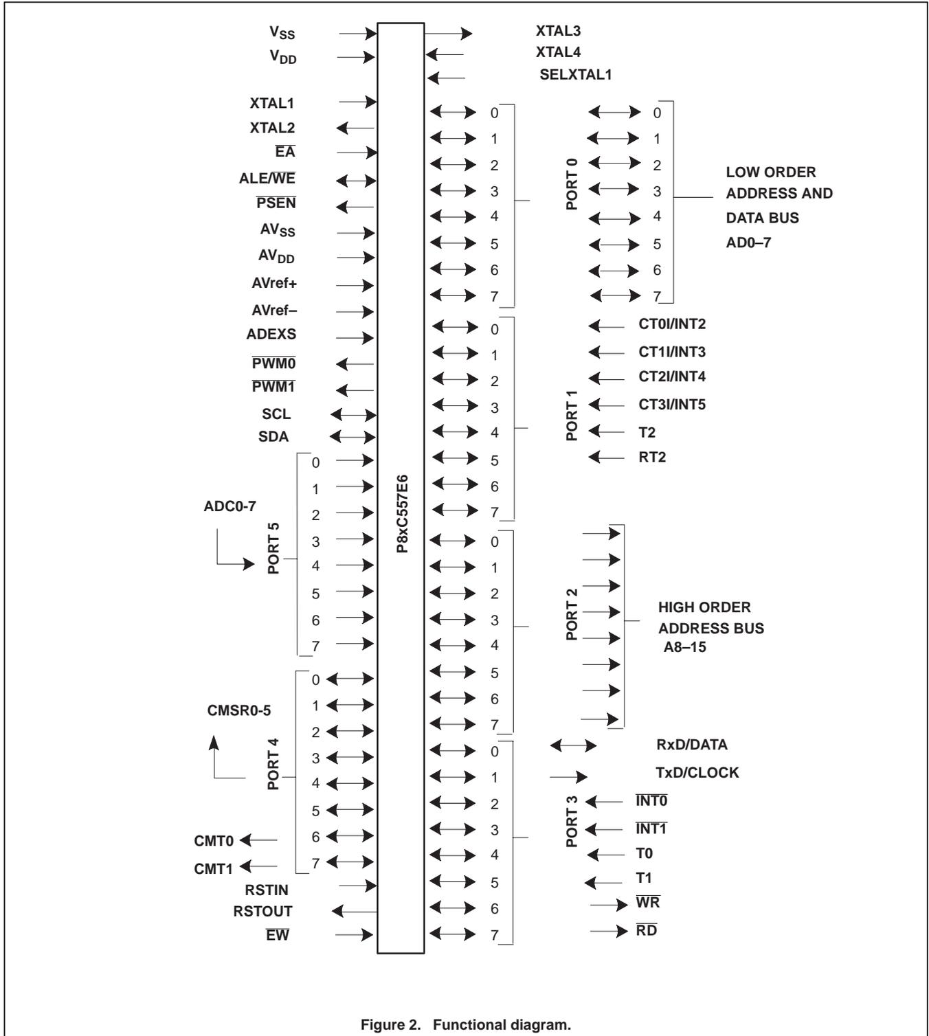
Figure 2. Functional diagram.
