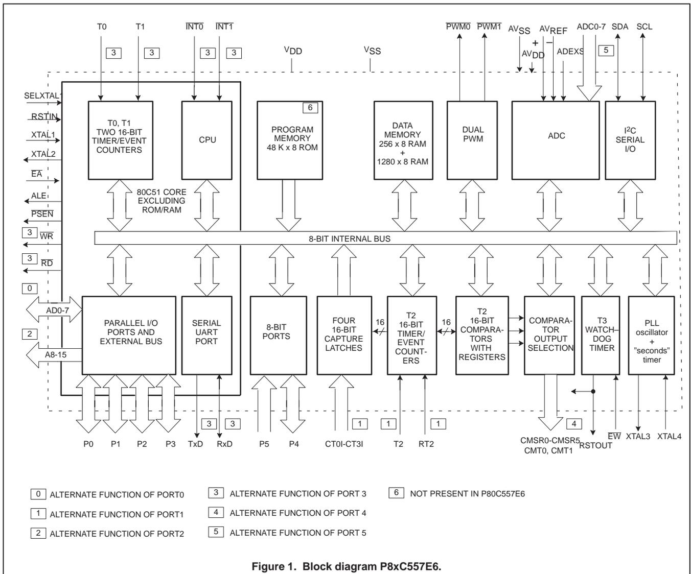
Figure 1. Block diagram P8xC557E6.
