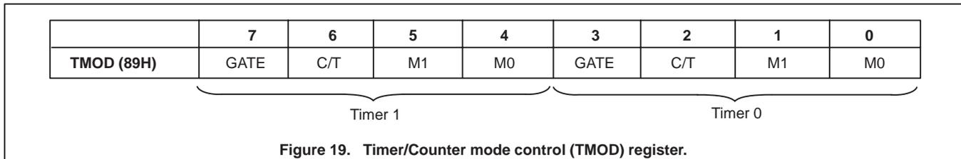
Figure 19. Timer/Counter mode control (TMOD) register.
