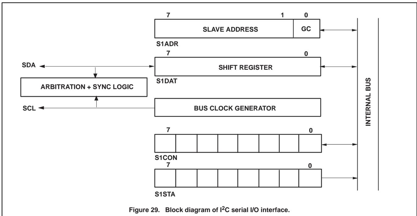
Figure 29. Block diagram of I<sup>2</sup>C serial I/O interface.
