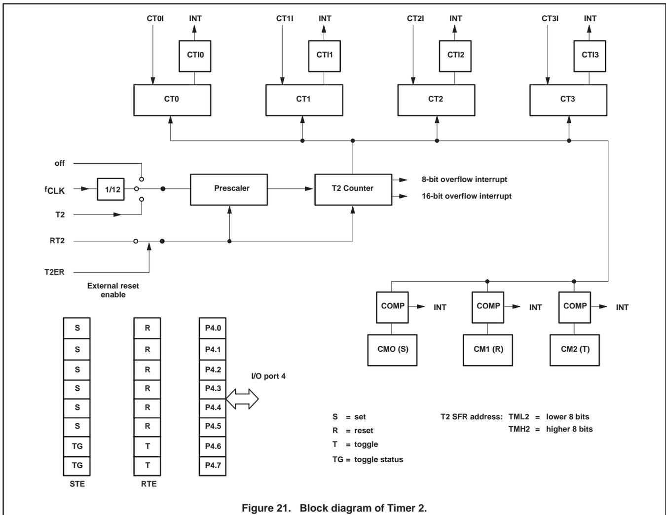
Figure 21. Block diagram of Timer 2.
