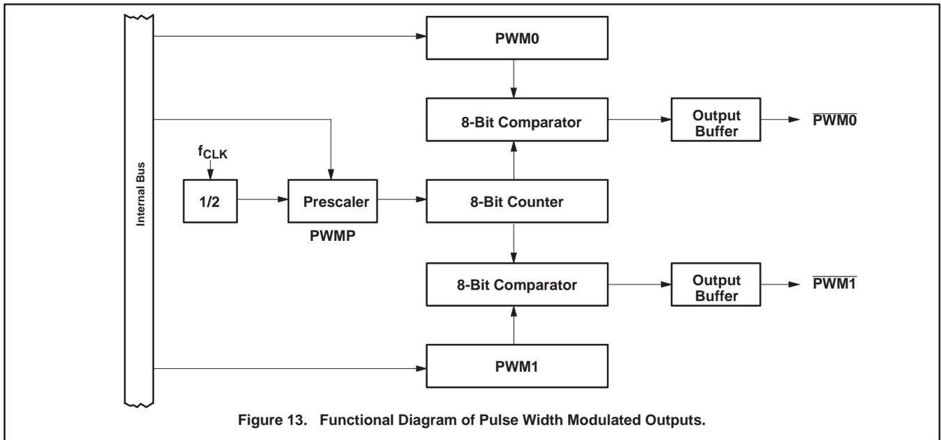
Figure 13. Functional Diagram of Pulse Width Modulated Outputs.
