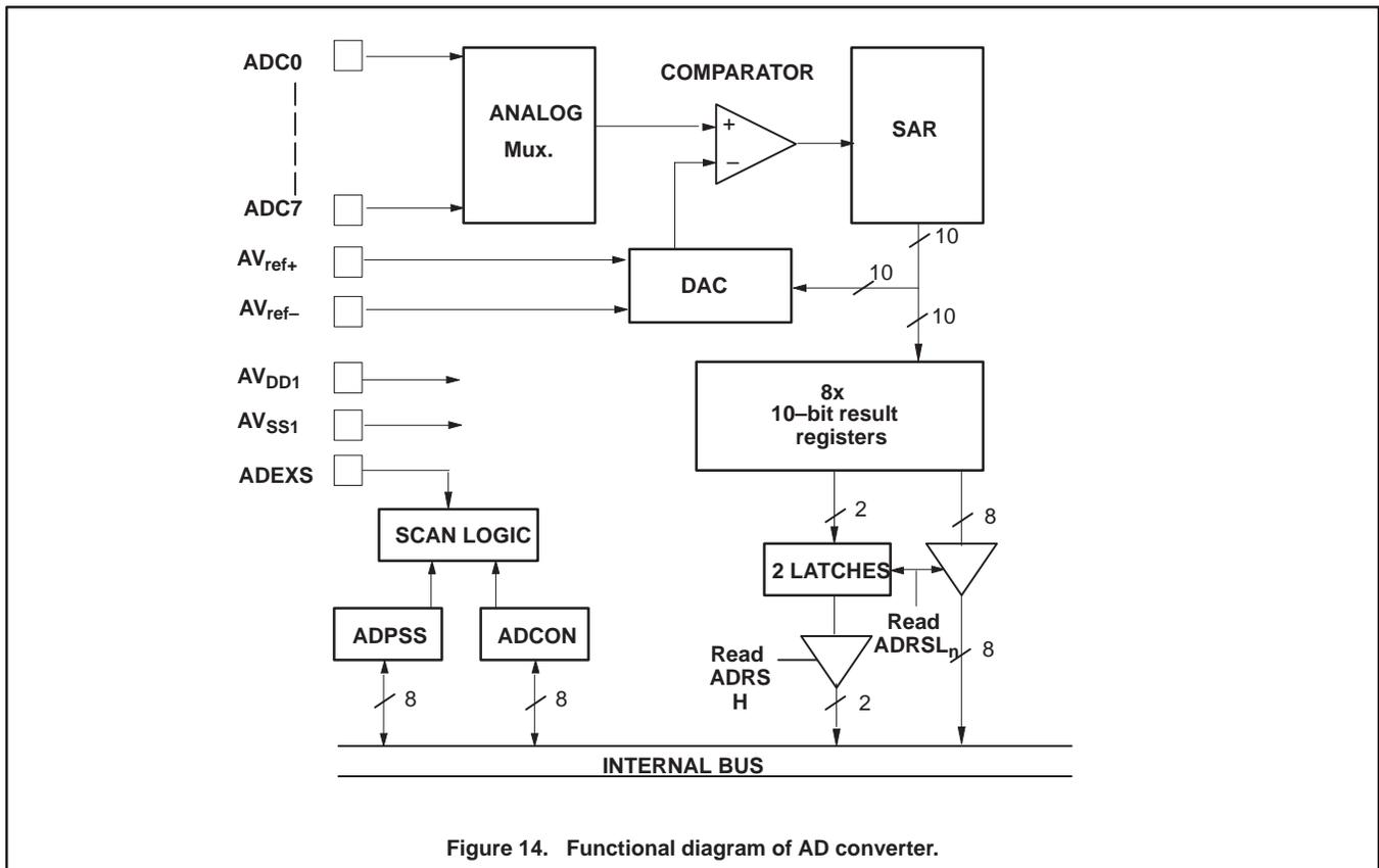
Figure 14. Functional diagram of AD converter.
