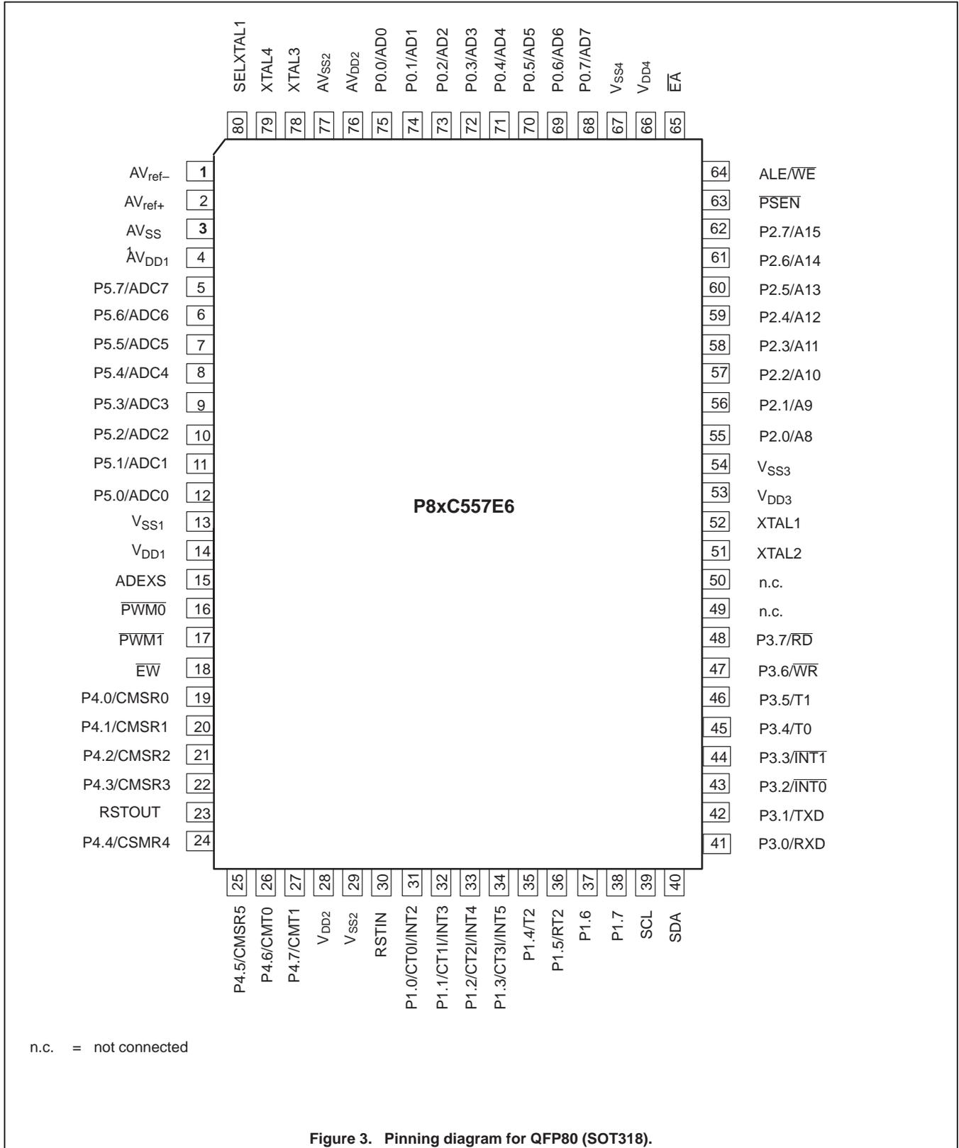
Figure 3. Pinning diagram for QFP80 (SOT318).
