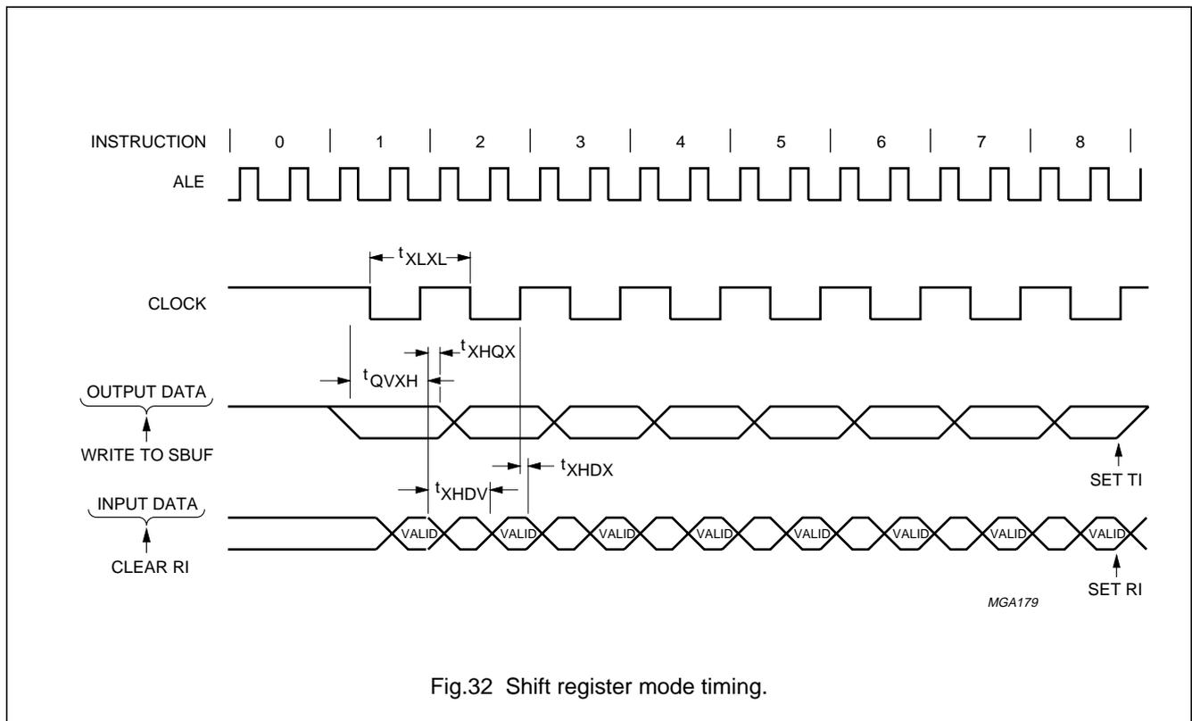
Fig.32 Shift register mode timing.
