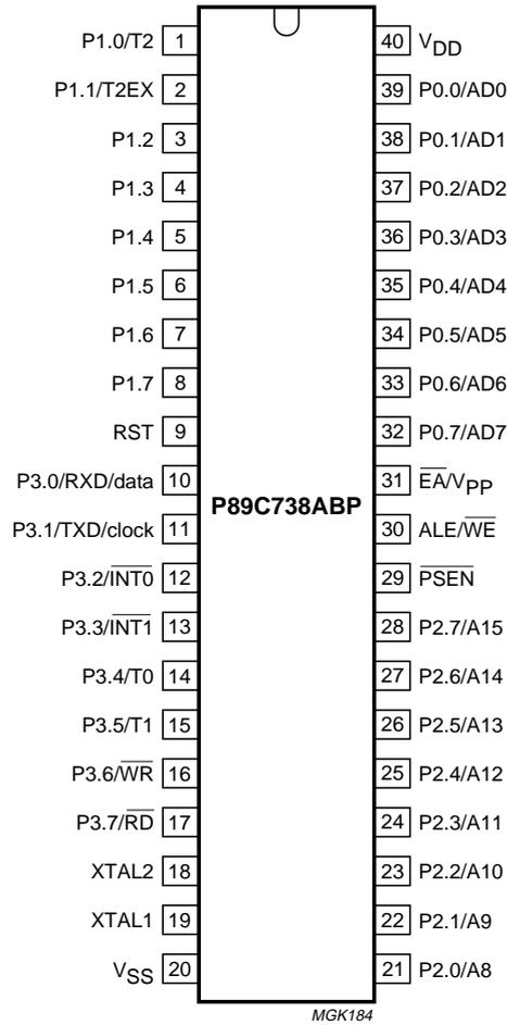
Fig.4 Pin configuration for DIP40 package (SOT129-1).
