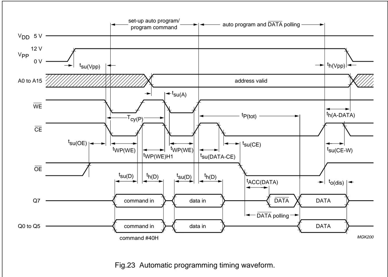
Fig.23 Automatic programming timing waveform.
