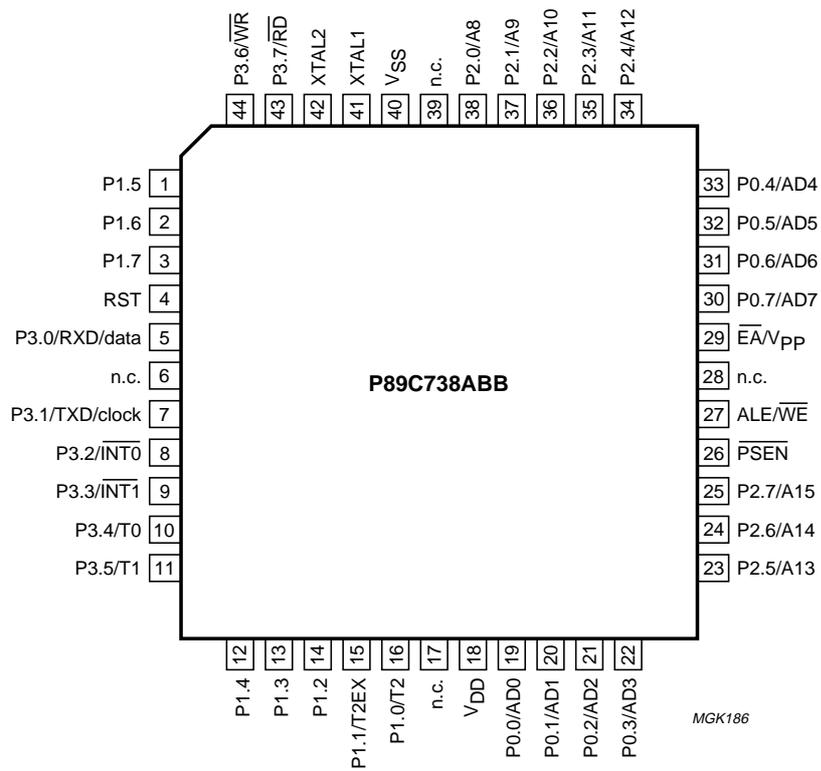
Fig.5 Pin configuration for QFP44 package; for more information on the version see Chapter 3.
