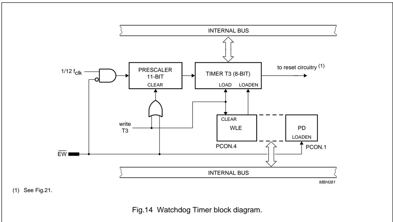
Fig.14 Watchdog Timer block diagram.
