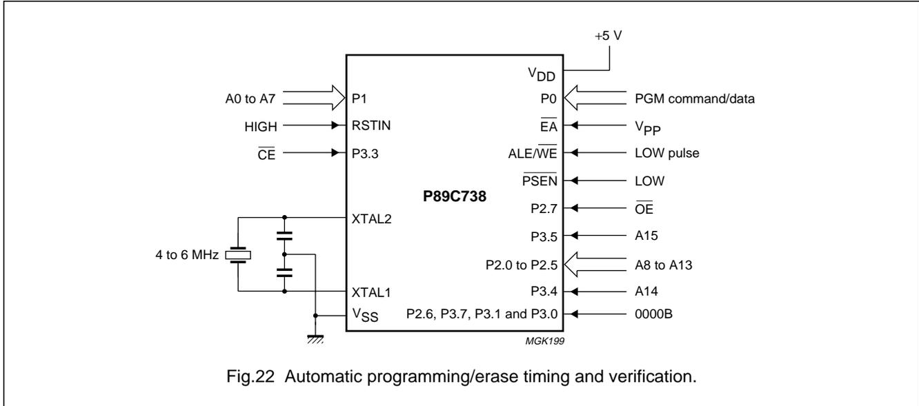
Fig.22 Automatic programming/erase timing and verification.
