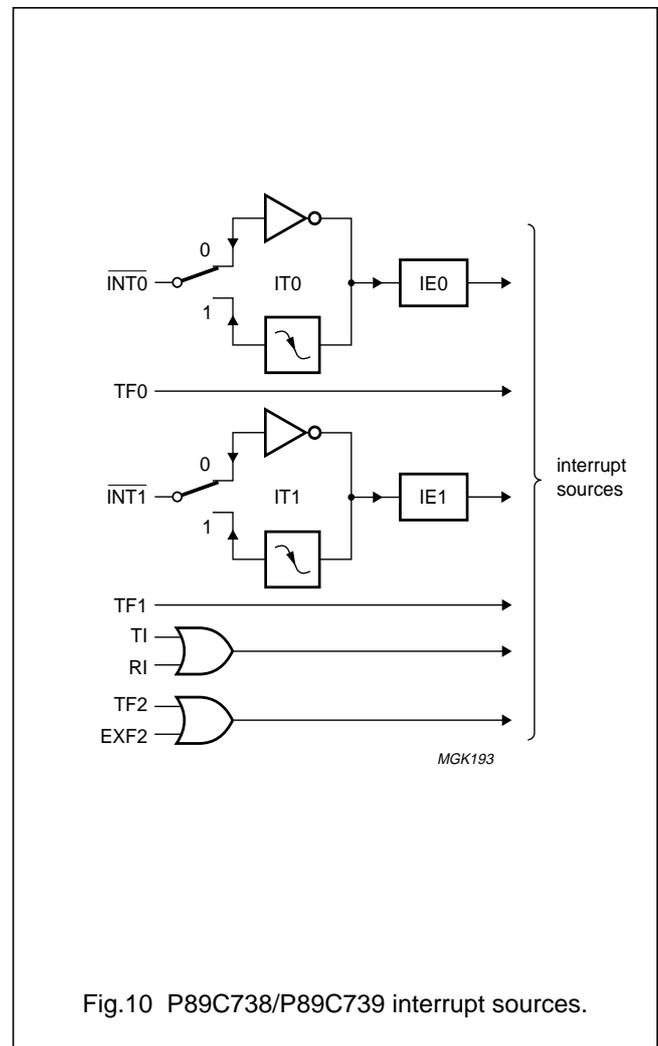
Fig.10 P89C738/P89C739 interrupt sources.
