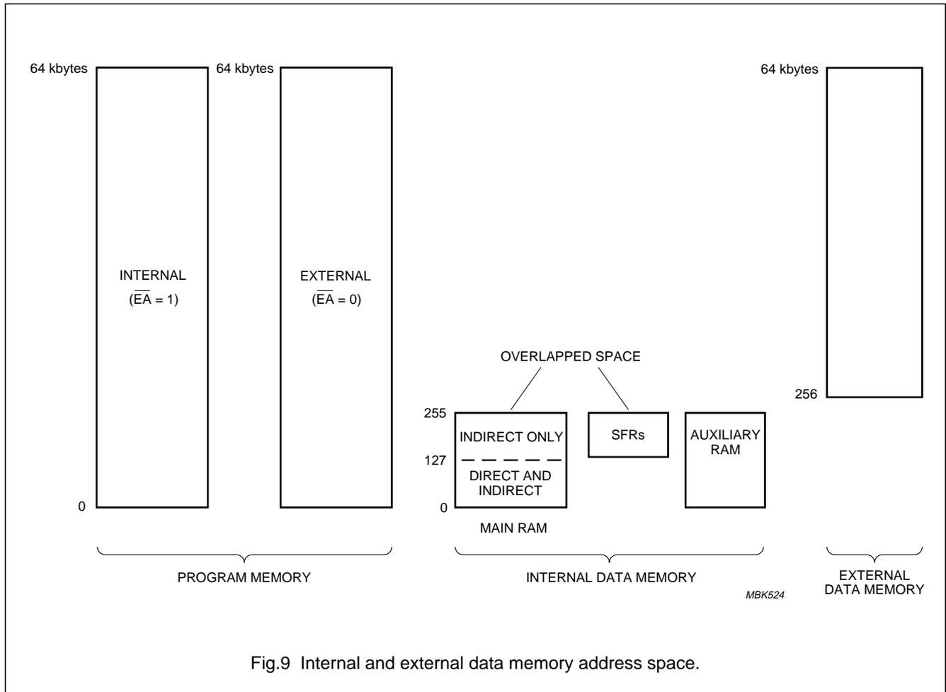
Fig.9 Internal and external data memory address space.
