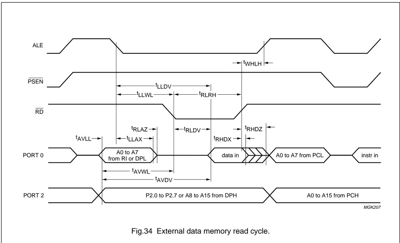
Fig.34 External data memory read cycle.
