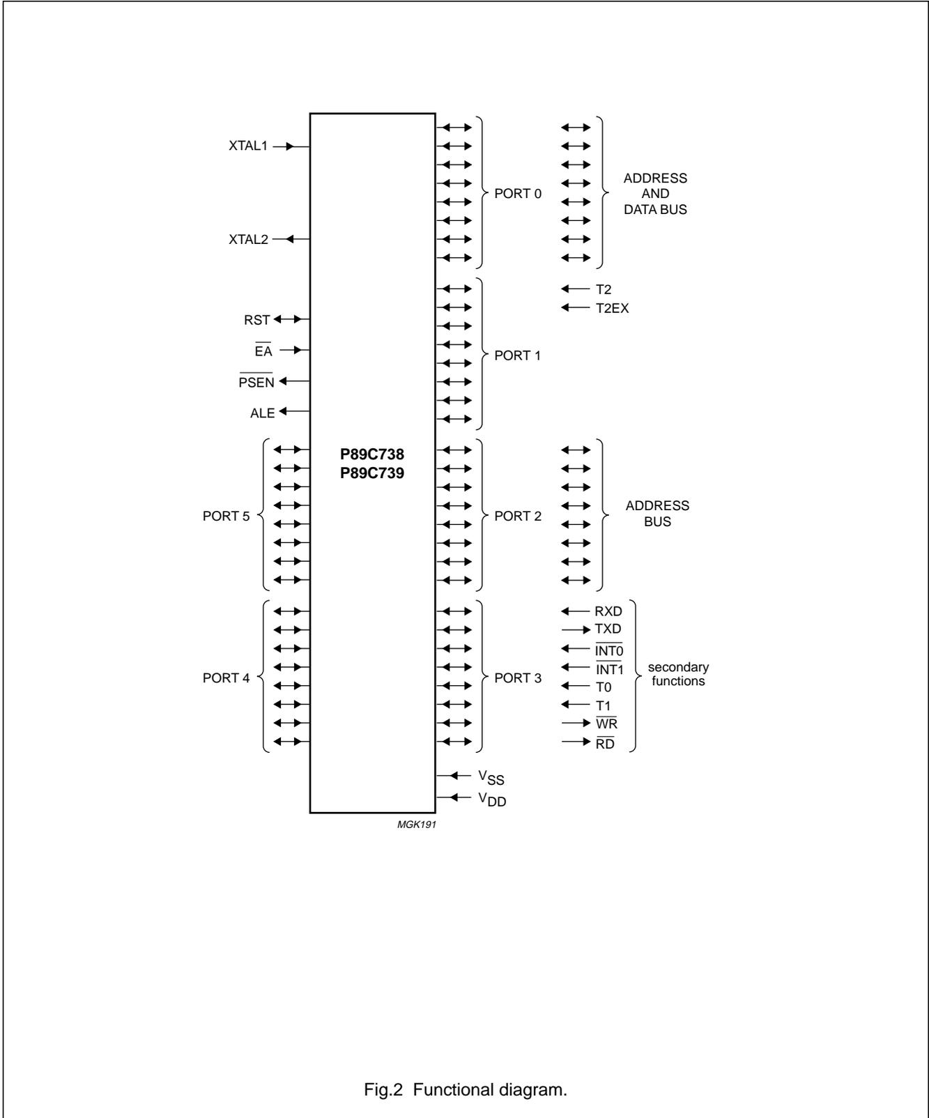
Fig.2 Functional diagram.
