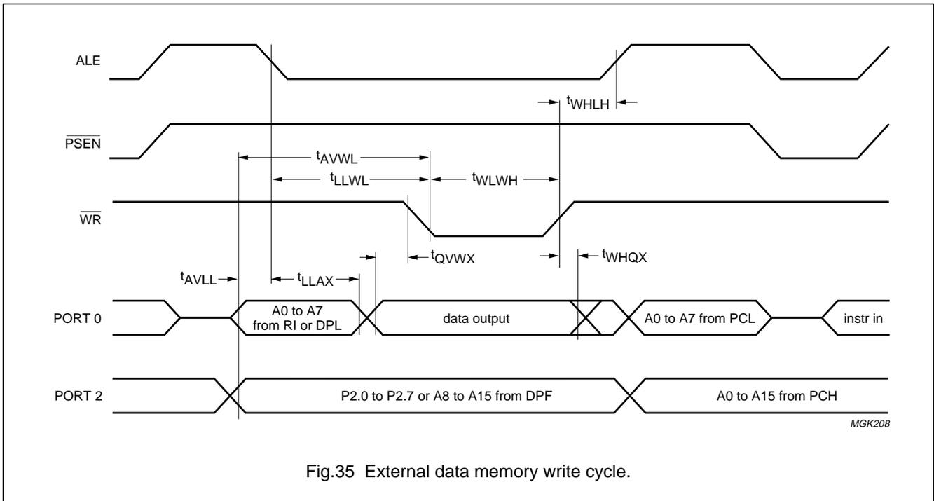
Fig.35 External data memory write cycle.
