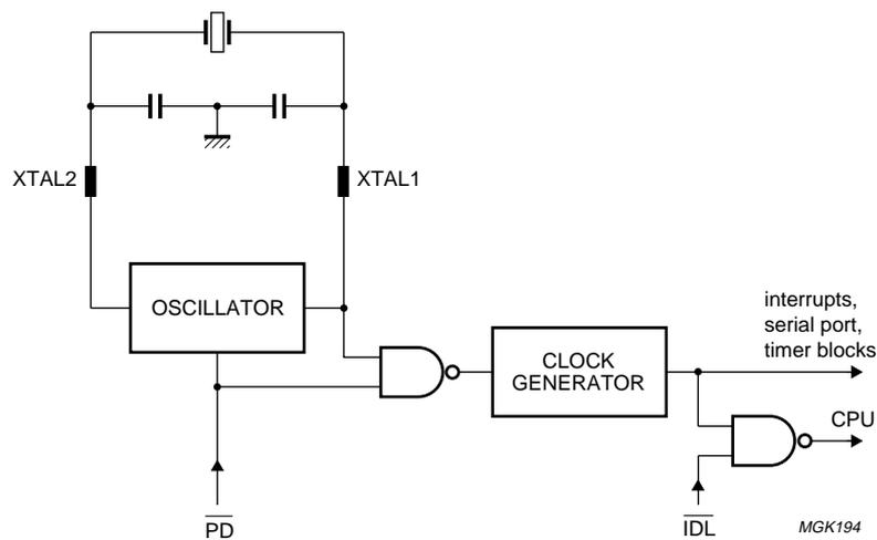
Fig.17 Internal Idle and Power-down clock configuration.
