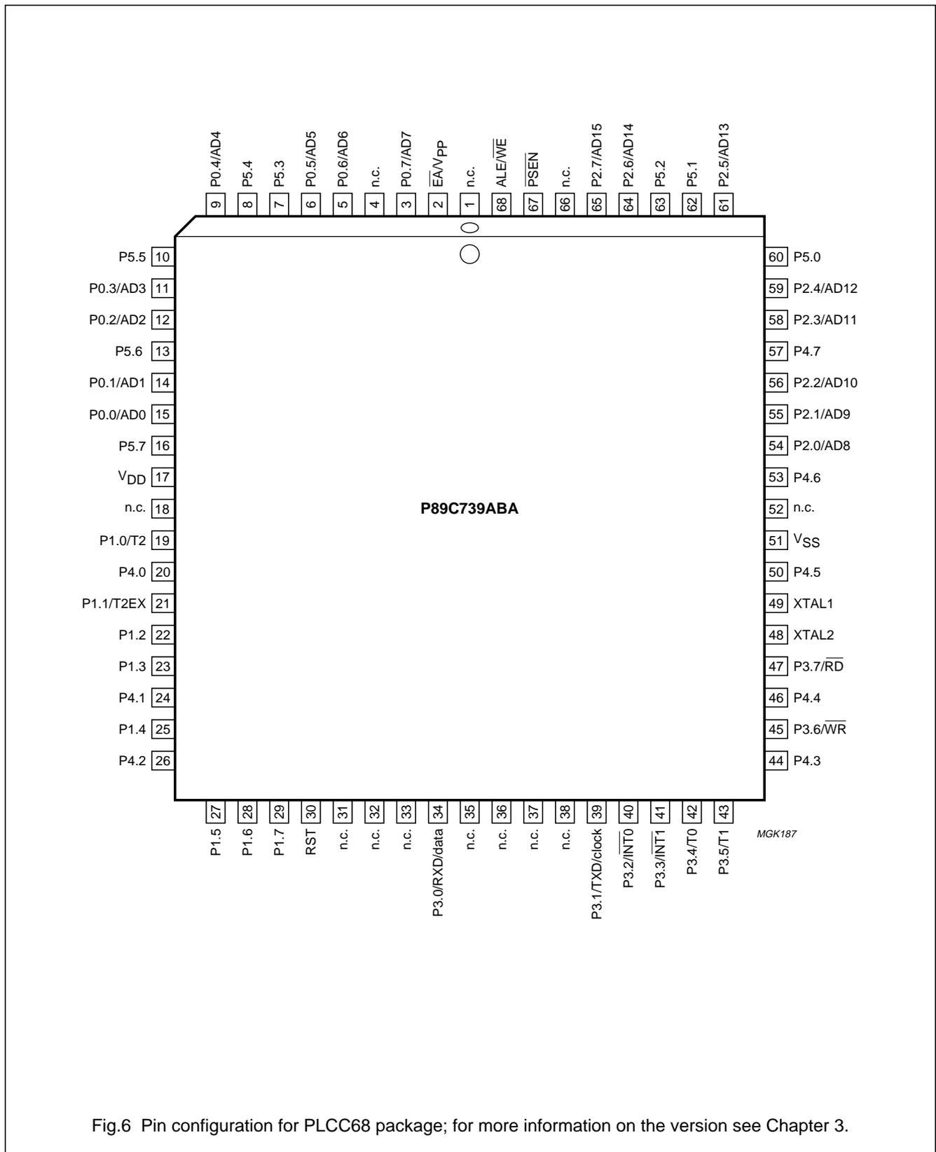
Fig.6 Pin configuration for PLCC68 package; for more information on the version see Chapter 3.
