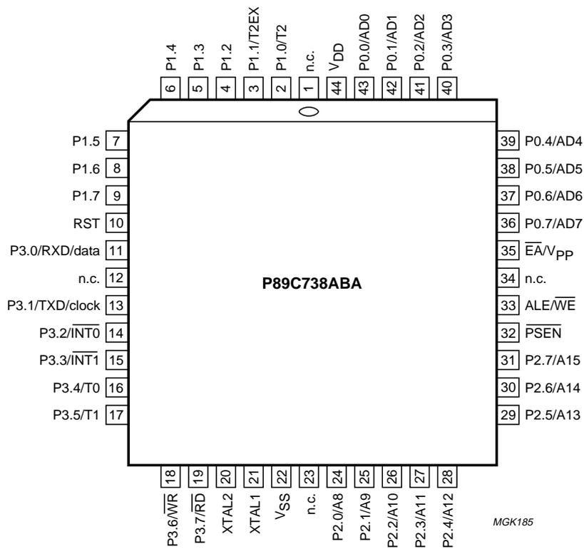
Fig.3 Pin configuration for PLCC44 package; for more information on the version see Chapter 3.
