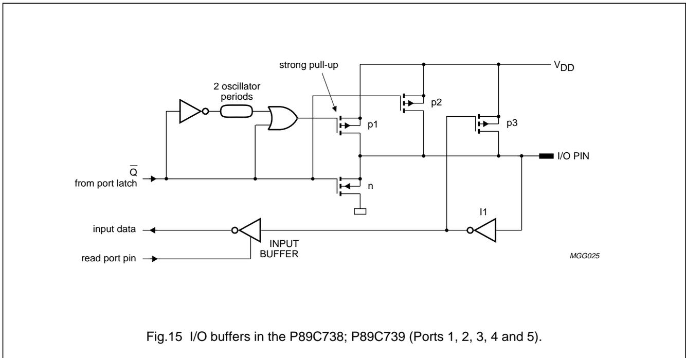
Fig.15 I/O buffers in the P89C738; P89C739 (Ports 1, 2, 3, 4 and 5).
