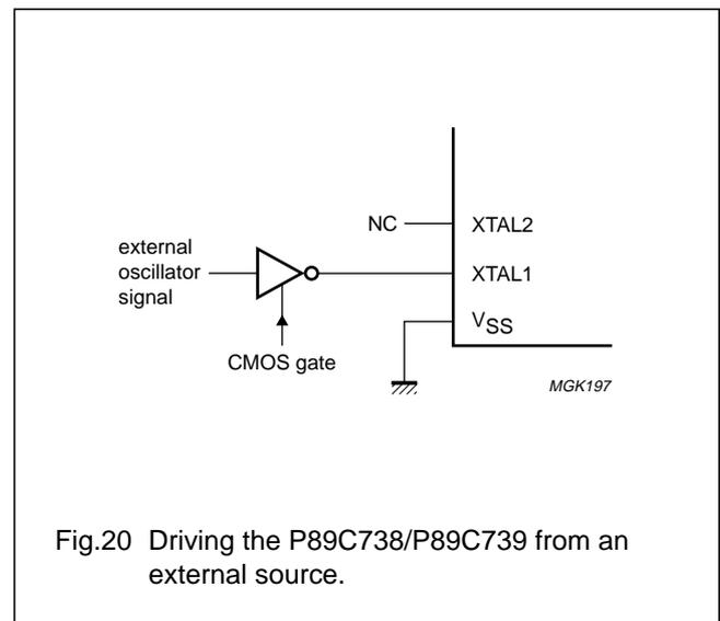
Fig.20 Driving the P89C738/P89C739 from an external source.
