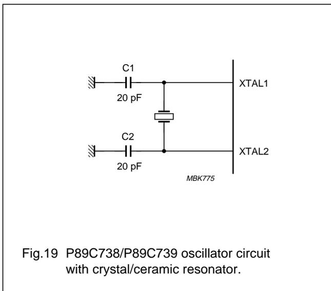
Fig.19 P89C738/P89C739 oscillator circuit with crystal/ceramic resonator.
