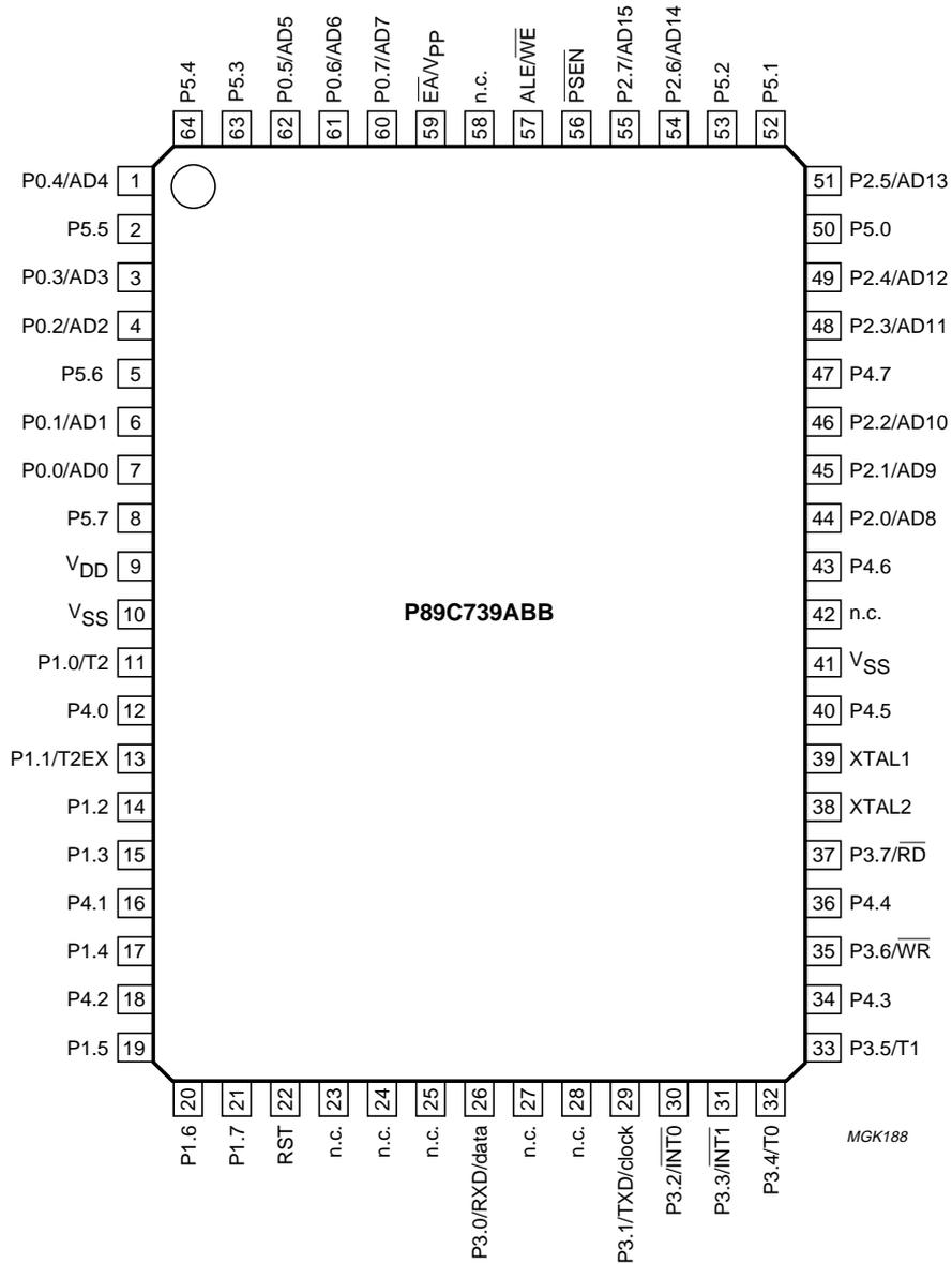
Fig.7 Pin configuration for QFP64 package (SOT319-1).
