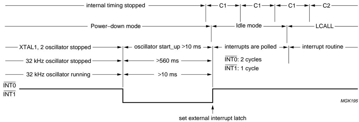
Fig.16 Wake-up by external interrupt input.
