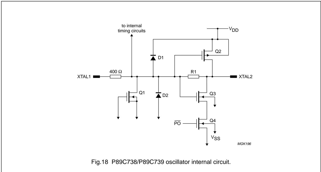
Fig.18 P89C738/P89C739 oscillator internal circuit.
