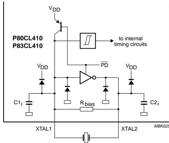
Fig.15 Standard oscillator.
