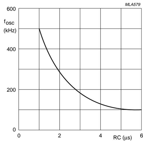
RC oscillator frequency is externally adjustable;  $100 \text{ kHz} \leq f_{osc} \leq 500 \text{ kHz}$ .
