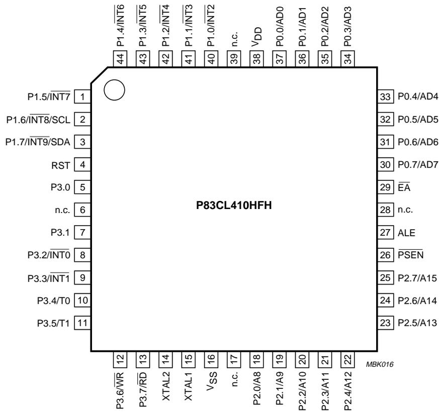
Fig.4 Pin configuration for QFP44 package.
