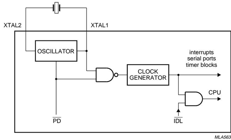
Fig.9 Internal clock control in Idle and Power-down mode.
