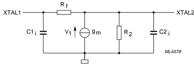
Fig.17 Oscillator equivalent circuit diagram.
