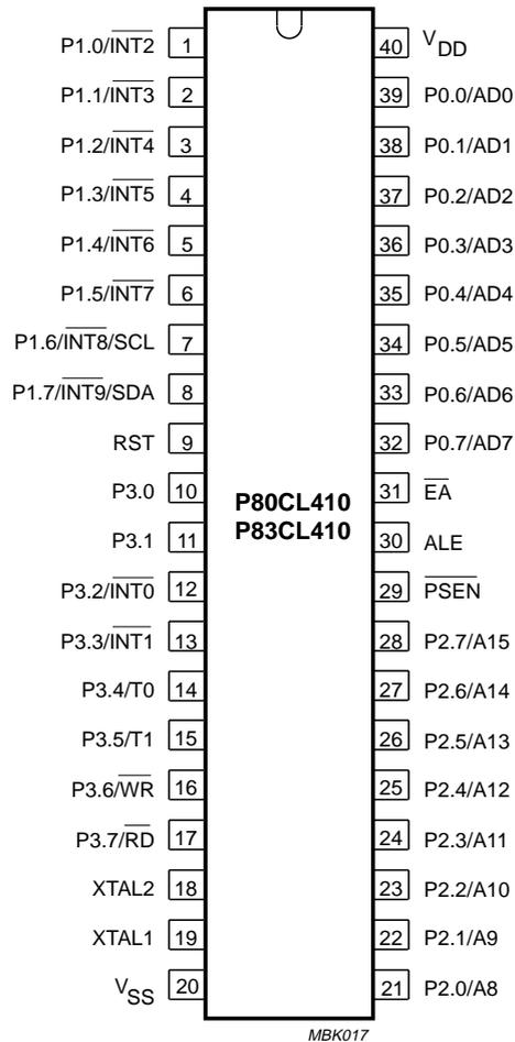
Fig.3 Pin configuration for DIP40 and VSO40 packages.
