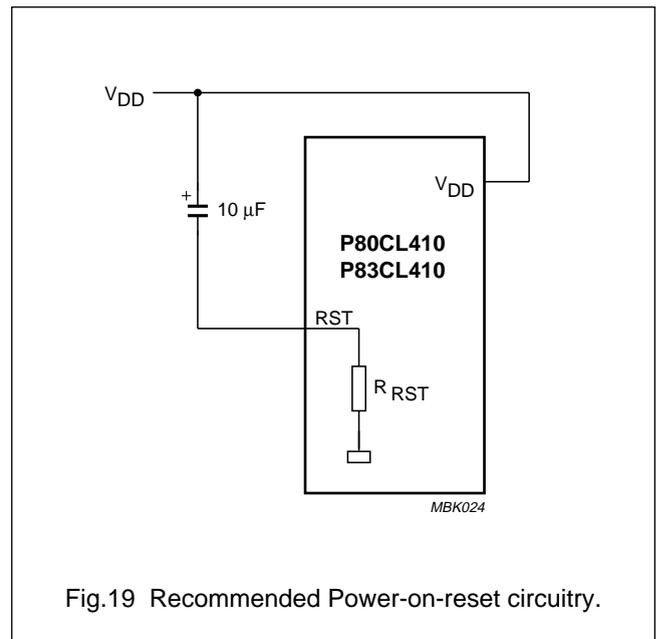
Fig.19 Recommended Power-on-reset circuitry.
