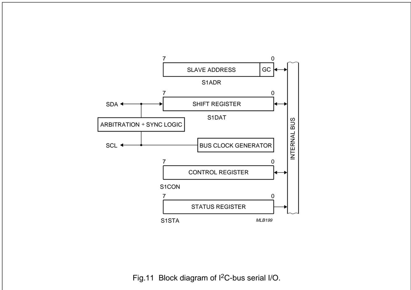
Fig.11 Block diagram of I<sup>2</sup>C-bus serial I/O.
