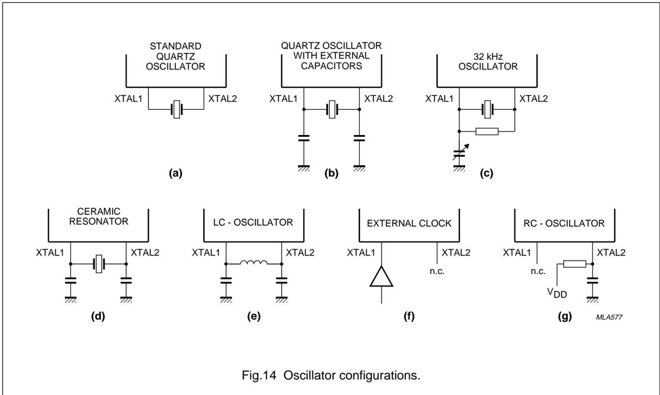
Fig.14 Oscillator configurations.
