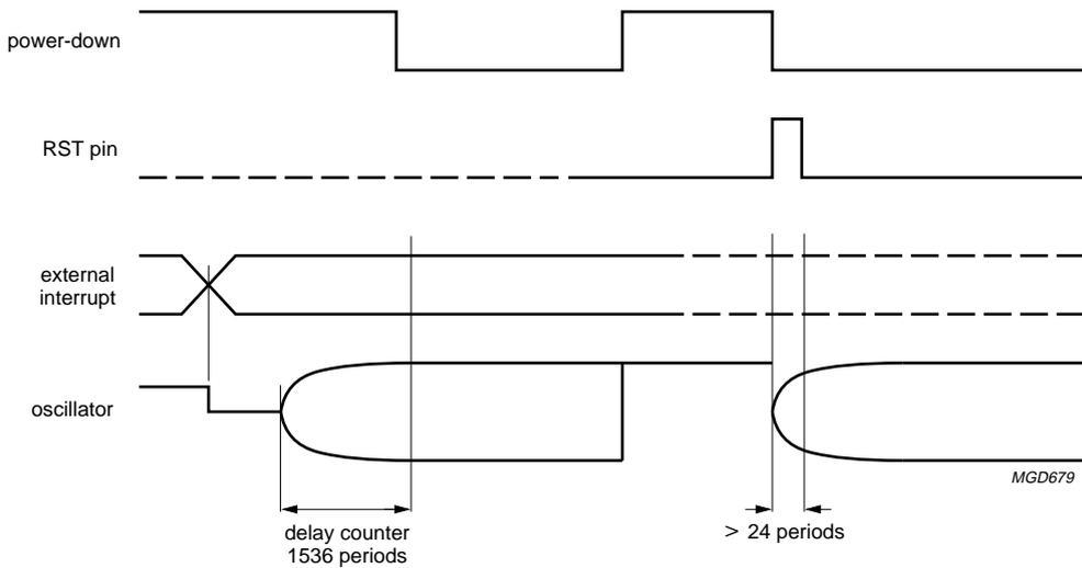
Fig.10 Wake-up operation.
