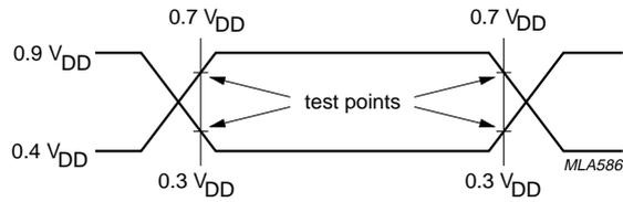
Fig.30 AC testing input waveform.
