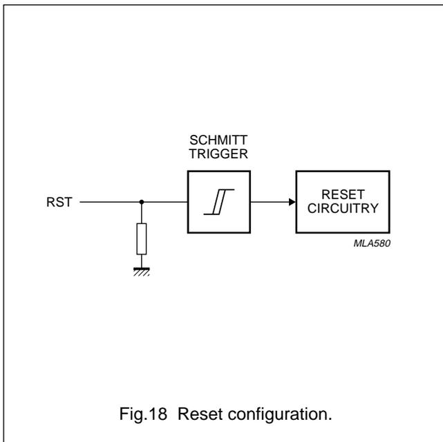
Fig.18 Reset configuration.
