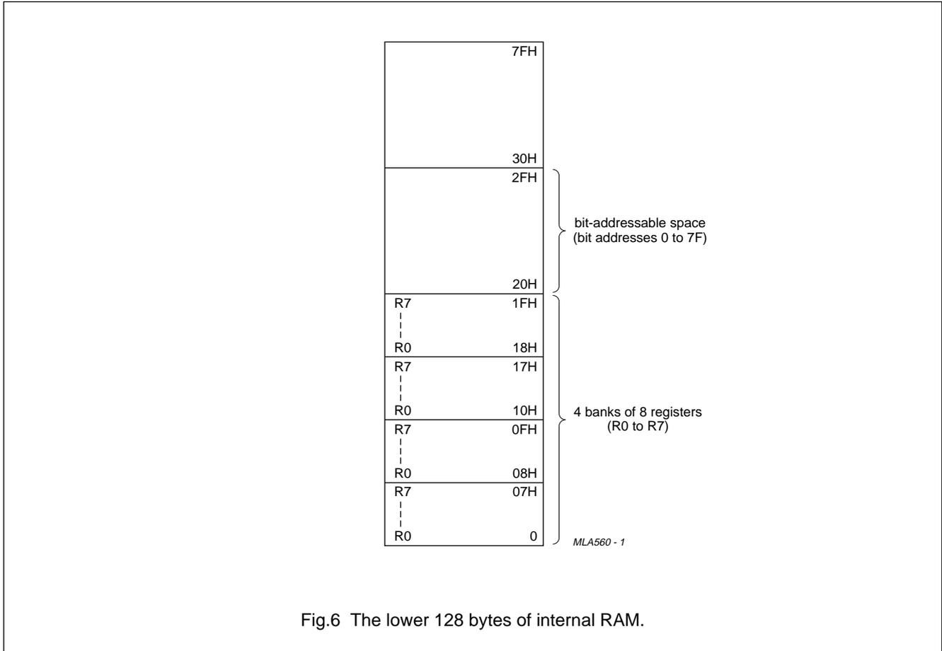
Fig.6 The lower 128 bytes of internal RAM.
