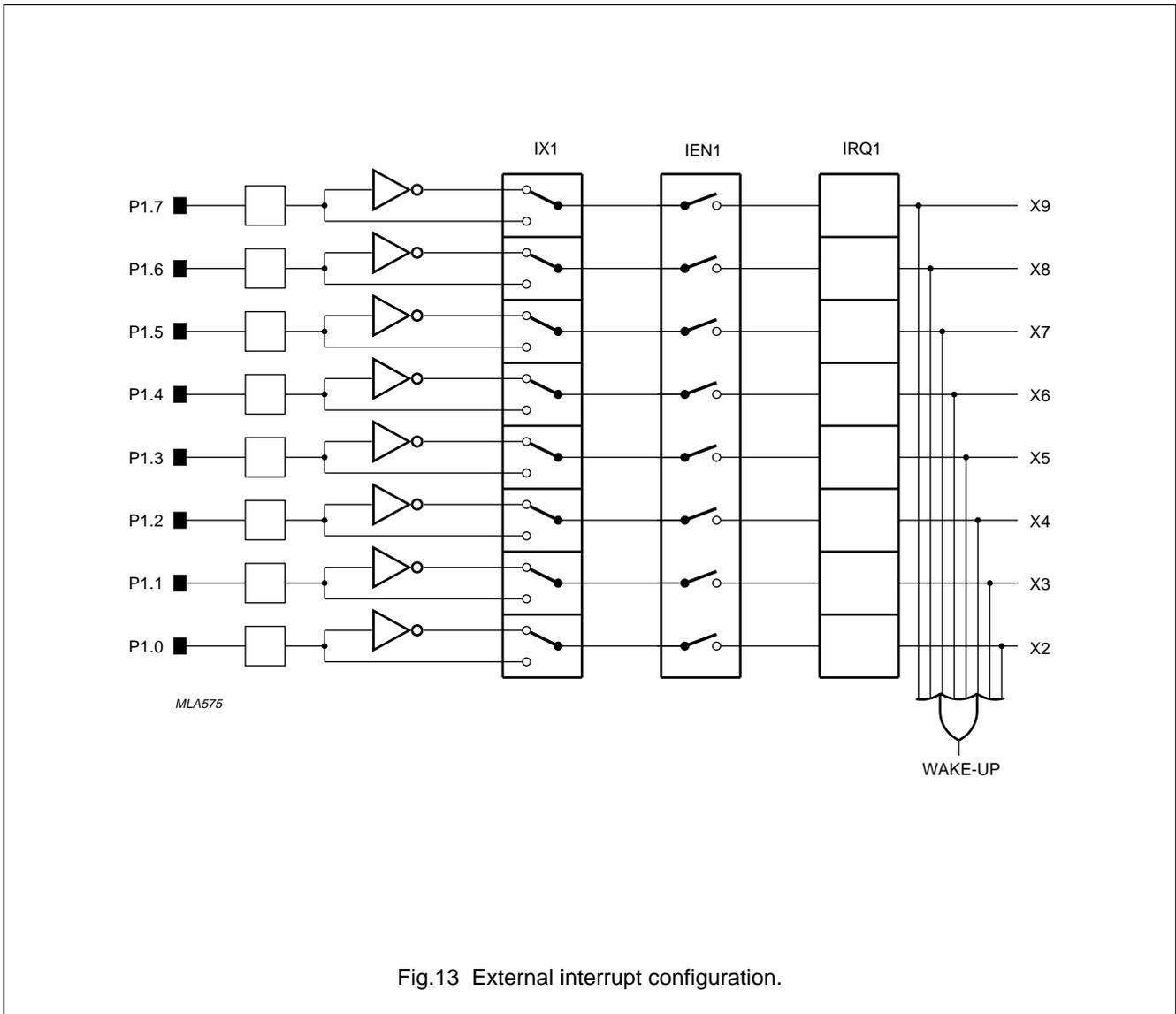
Fig.13 External interrupt configuration.
