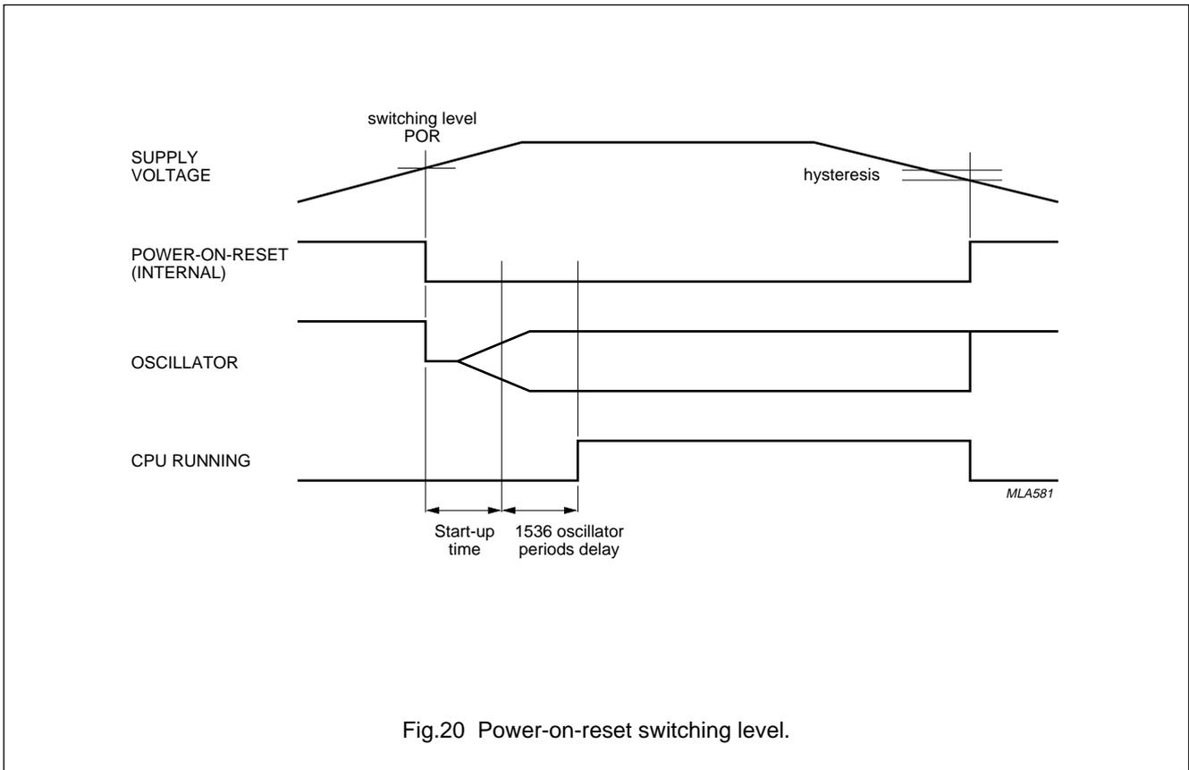
Fig.20 Power-on-reset switching level.
