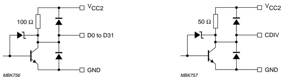
Fig.4 GTL output circuits.
