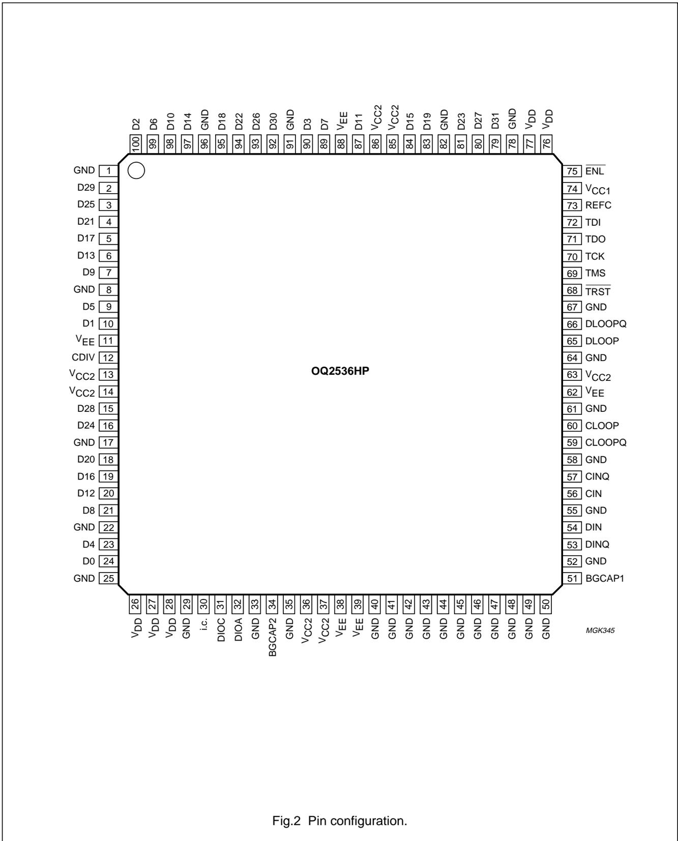
Fig.2 Pin configuration.
