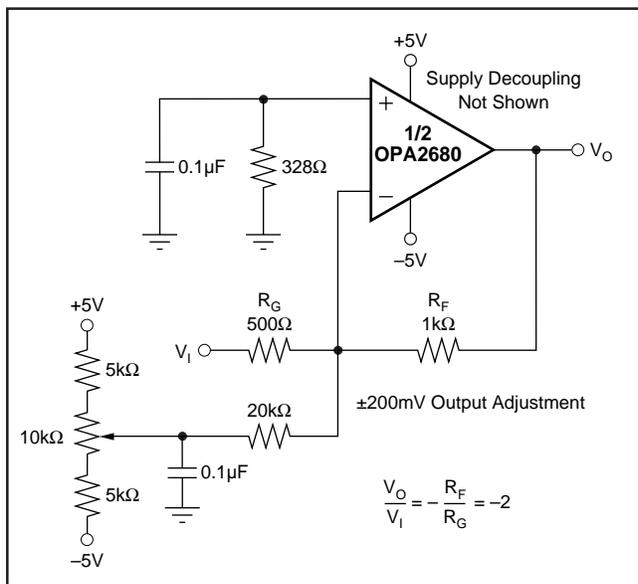
FIGURE 13. DC-Coupled, Inverting Gain of  $-2$ , with Offset Adjustment.
