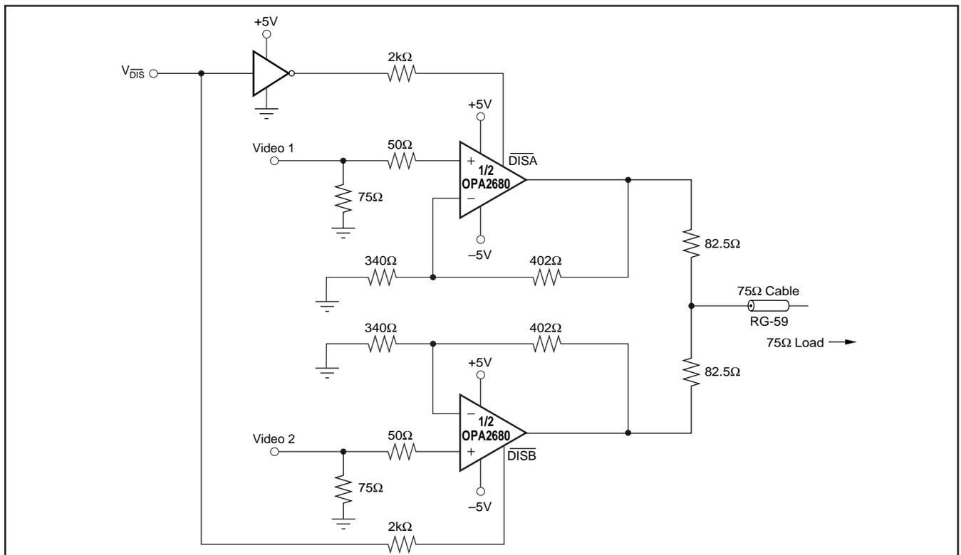
FIGURE 6. Two-Channel Video Multiplexer (SO-14 package only).
