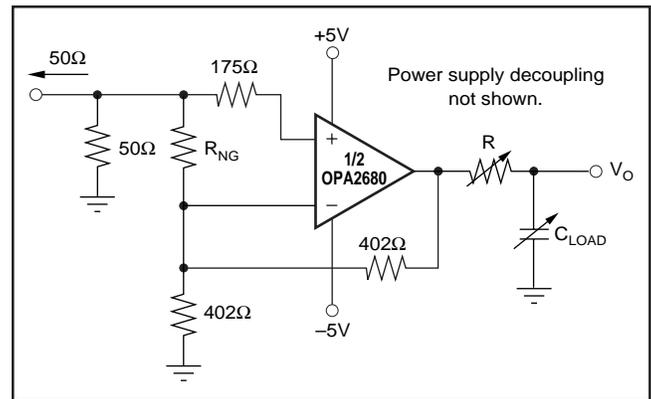
FIGURE 10. Capacitive Load Driving with Noise Gain Tuning.
