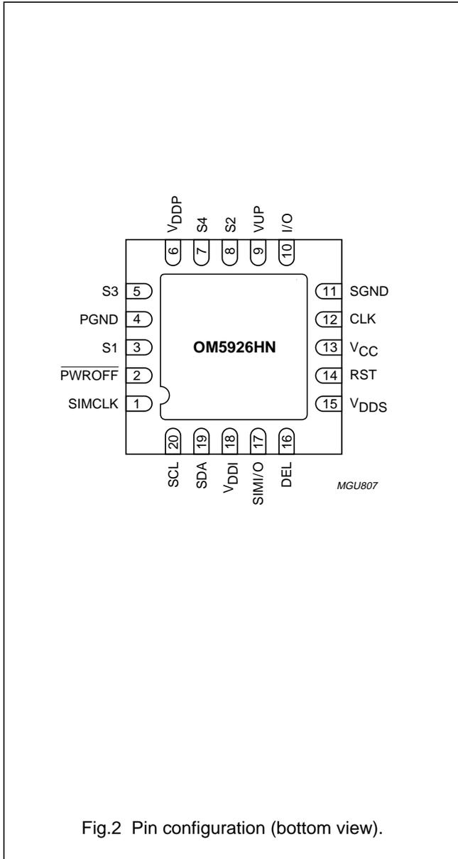
Fig.2 Pin configuration (bottom view).
