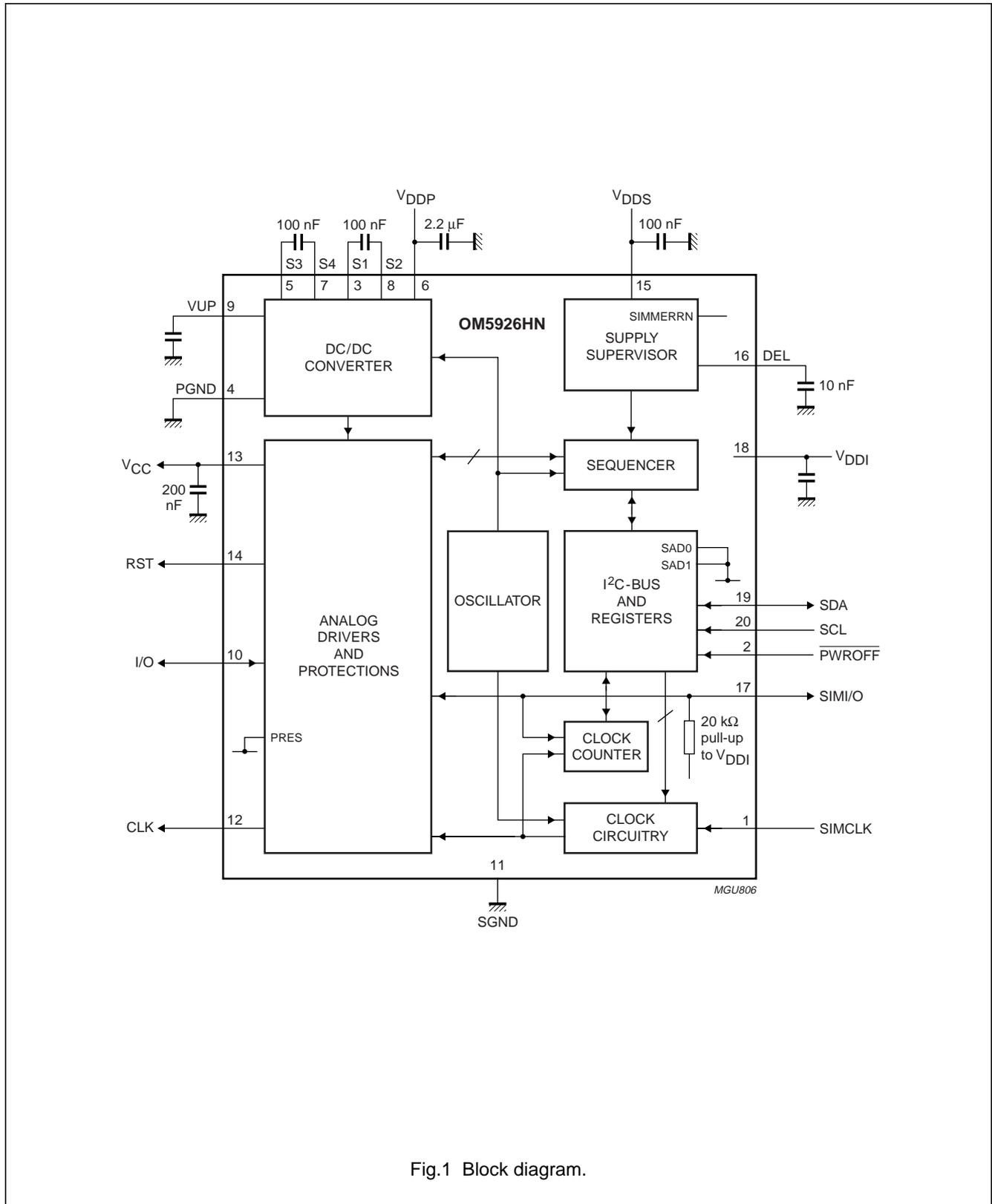
Fig.1 Block diagram.
