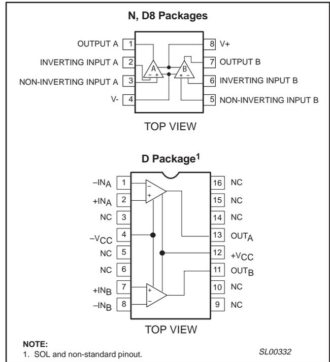
Figure 1. Pin Configurations
