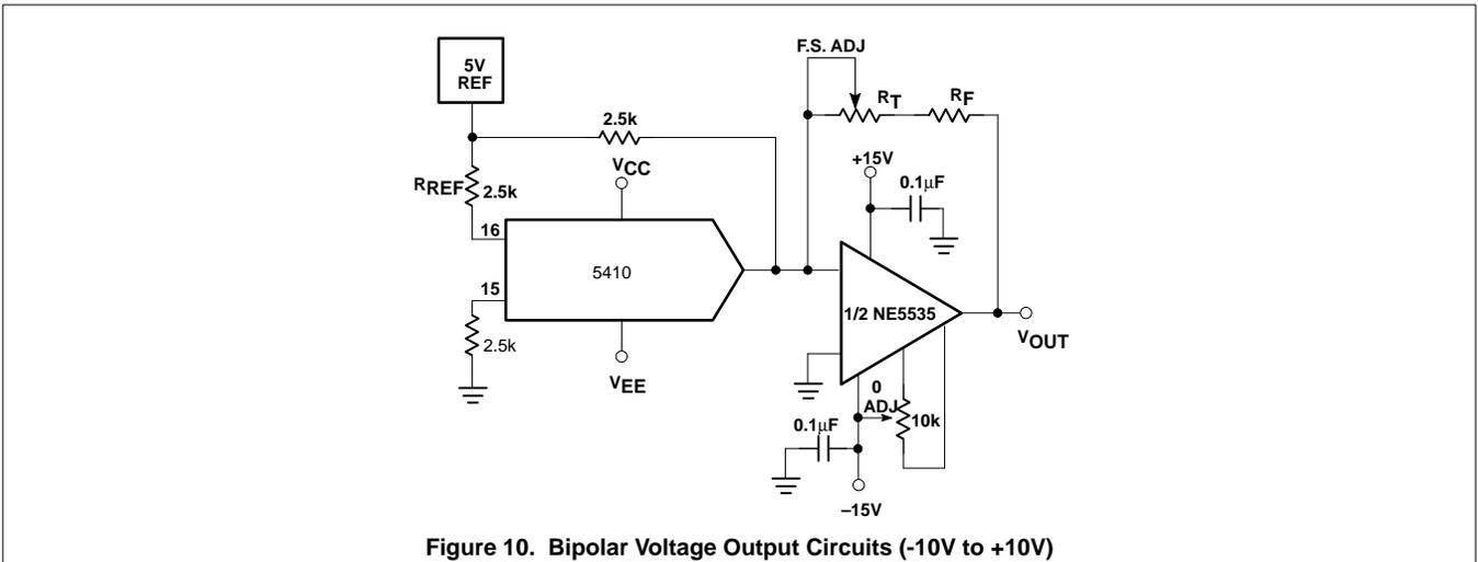
Figure 10. Bipolar Voltage Output Circuits (-10V to +10V)
