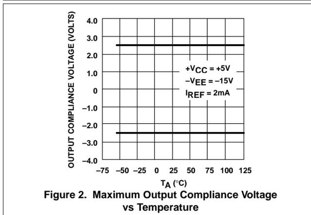
Figure 2. Maximum Output Compliance Voltage vs Temperature
