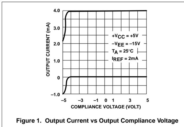
Figure 1. Output Current vs Output Compliance Voltage
