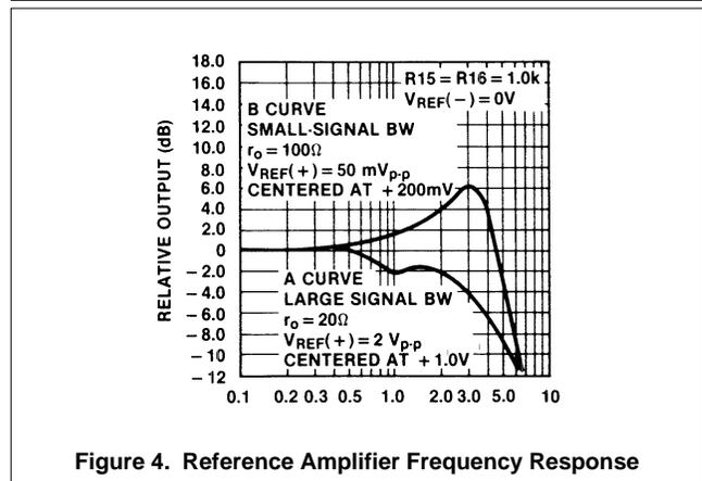
Figure 4. Reference Amplifier Frequency Response
