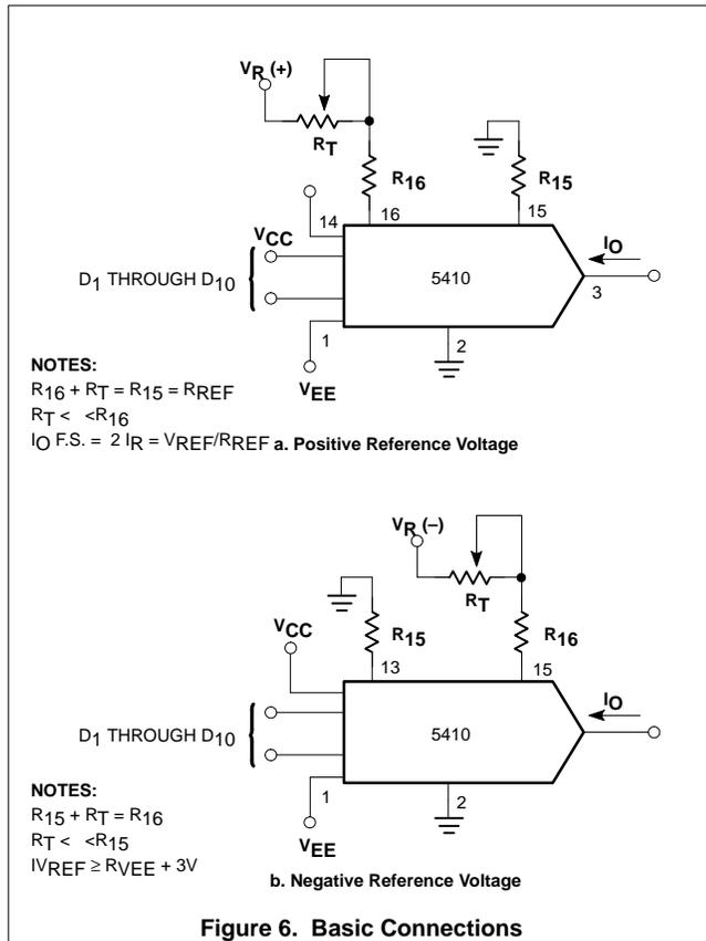
Figure 6. Basic Connections
