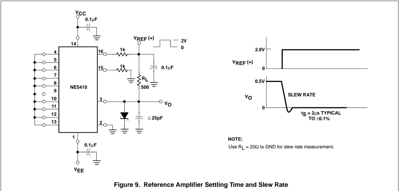
Figure 9. Reference Amplifier Settling Time and Slew Rate
