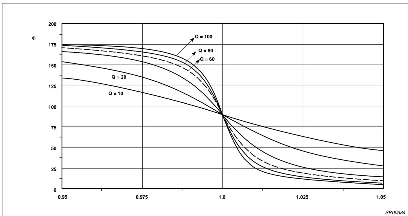
Figure 12. Phase vs Normalized IF Frequency  $\frac{\omega}{\omega_1} = 1 + \frac{\Delta\omega}{\omega_1}$
