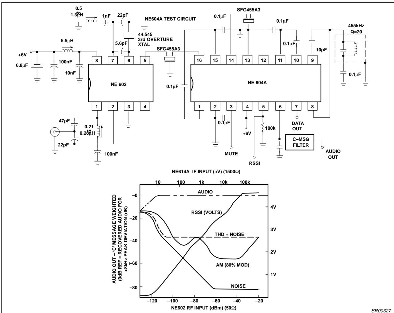
Figure 5. Typical Application Cellular Radio (45MHz to 455kHz)
