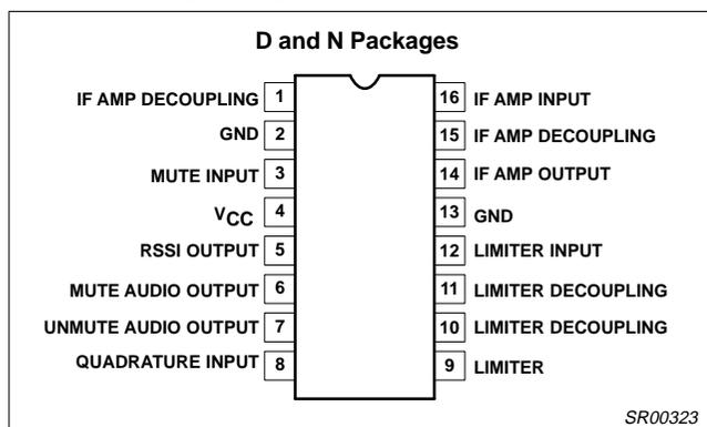
Figure 1. Pin Configuration
