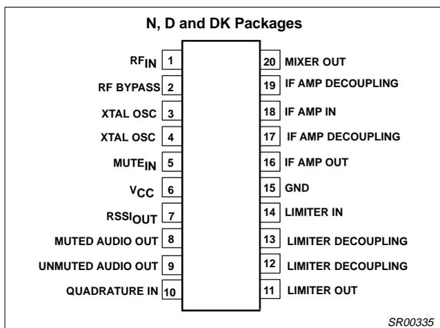
Figure 1. Pin Configuration
