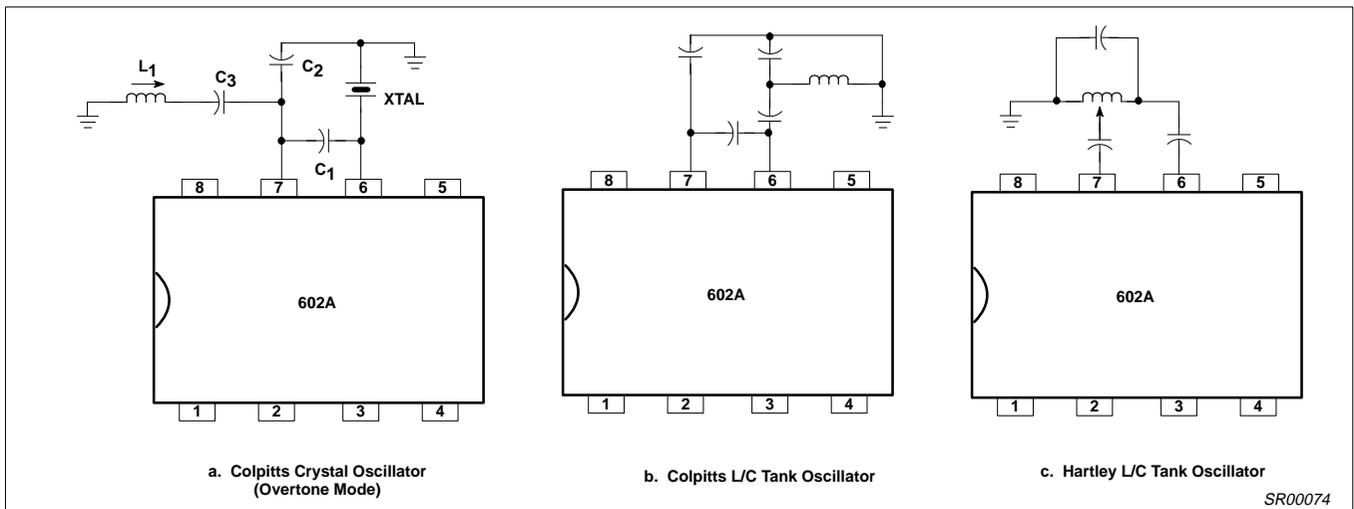
Figure 7. Oscillator Circuits
