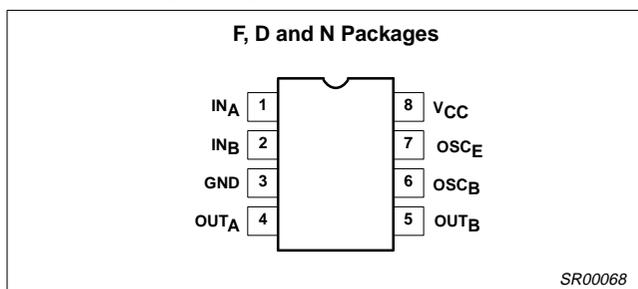
Figure 1. Pin Configuration
