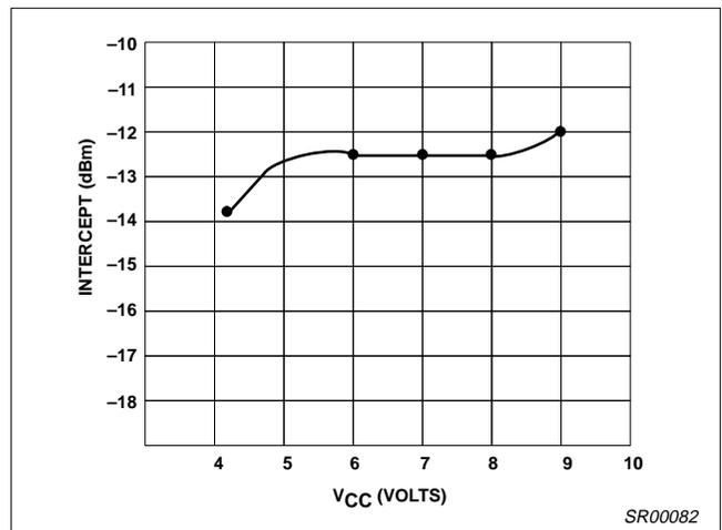
Figure 15. Input Third-Order Intermod Point vs  $V_{CC}$
