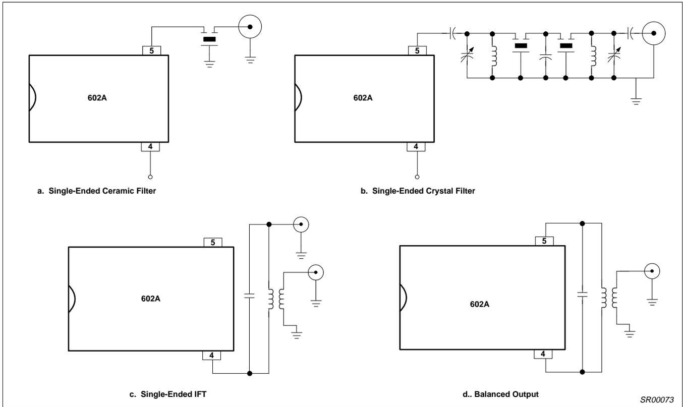
Figure 6. Output Configuration
