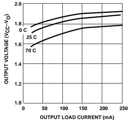
Output Voltage Drop vs Load Current (NE591)
