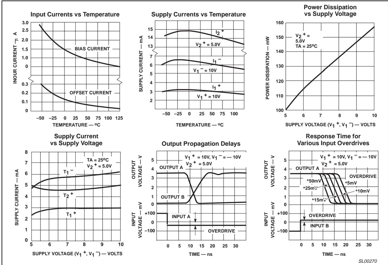
Figure 4. Typical Performance Characteristics
