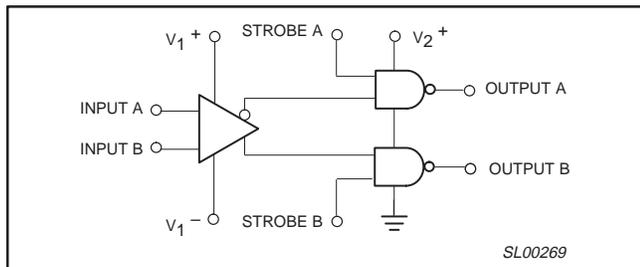
Figure 3. Block Diagram
