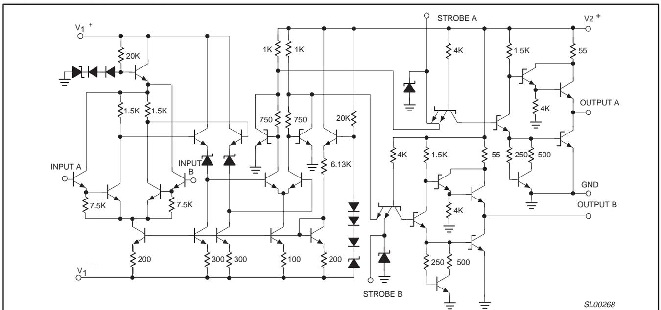
Figure 2. Equivalent Schematic
