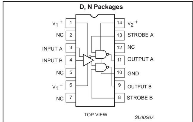
Figure 1. Pin Configuration
