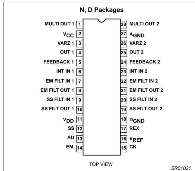
Figure 1. Pin Configuration
