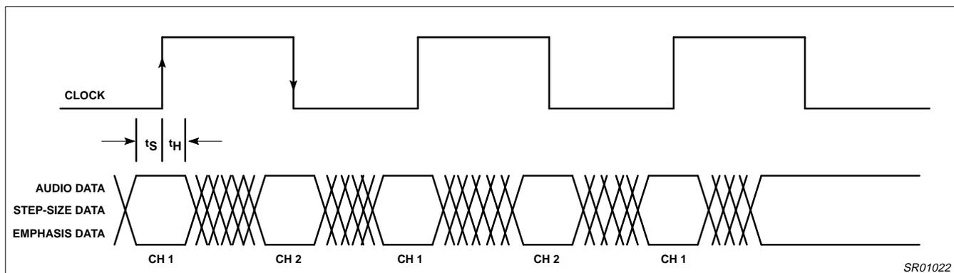
Figure 2. Timing Diagram
