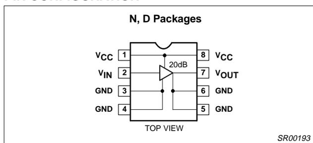
Figure 1. Pin Configuration
