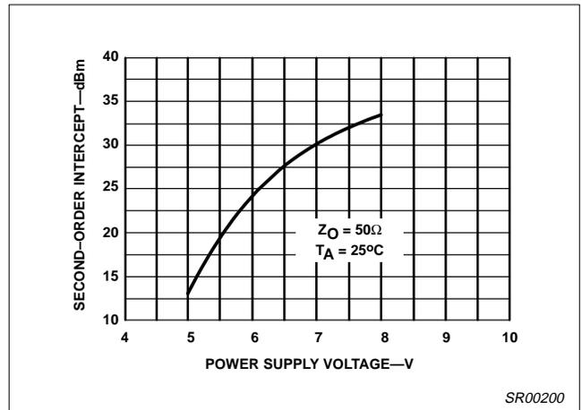
Figure 9. Second-Order Output Intercept vs Supply Voltage
