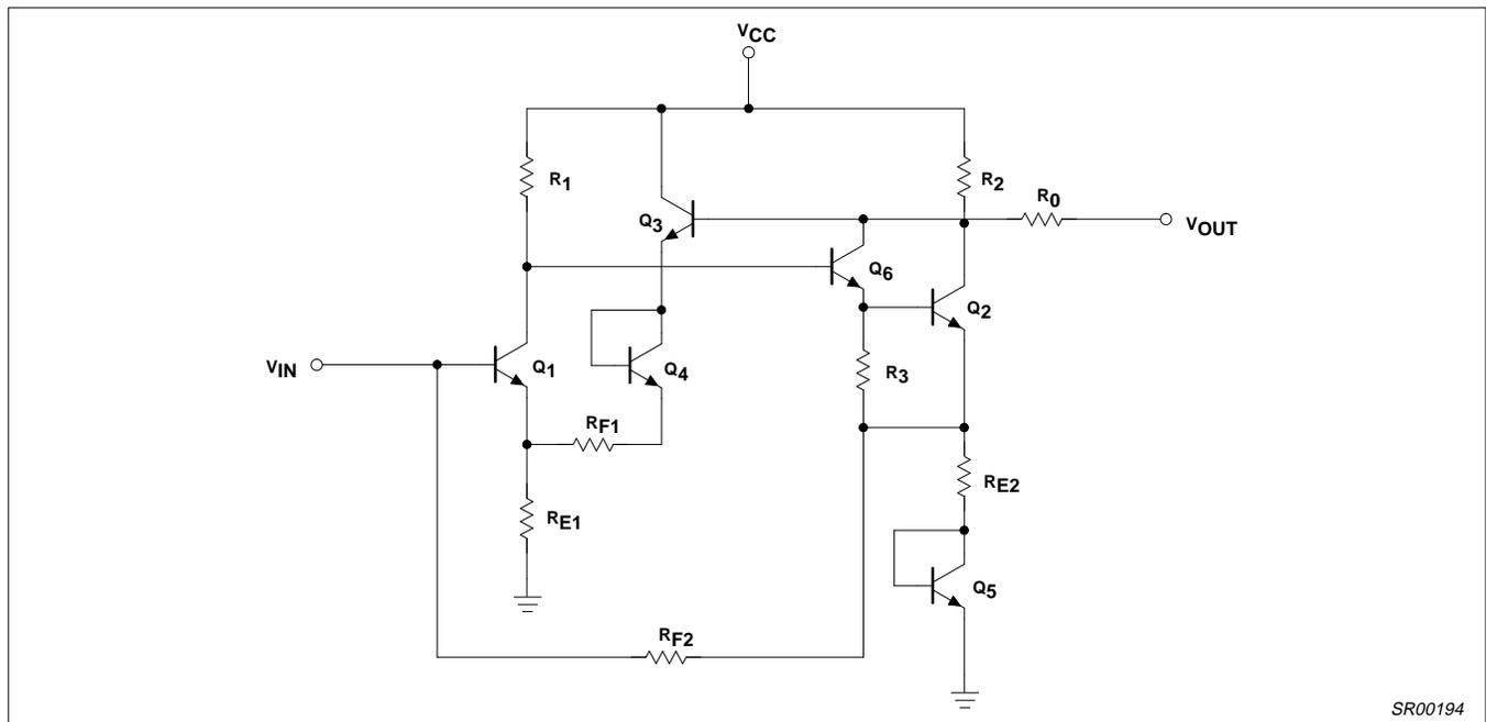
Figure 2. Equivalent Schematic
