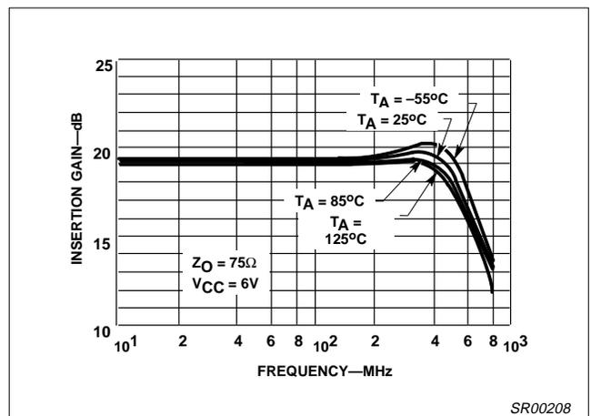
Figure 16. Insertion Gain vs Frequency ( $S_{21}$ )
