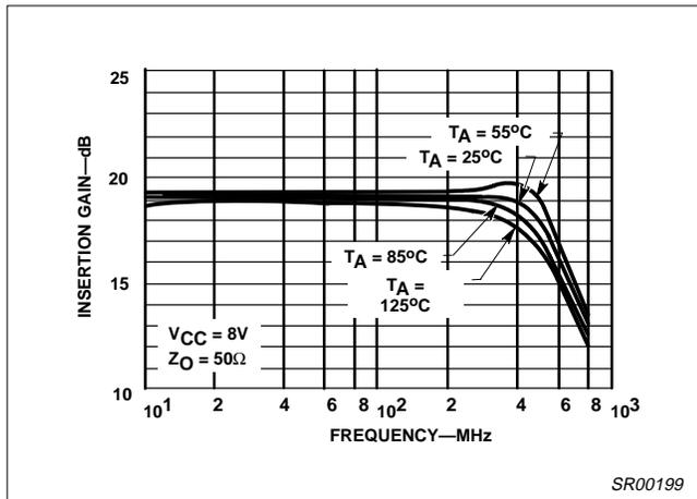
Figure 6. Insertion Gain vs Frequency ( $S_{21}$ )
