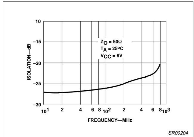
Figure 14. Isolation vs Frequency ( $S_{12}$ )
