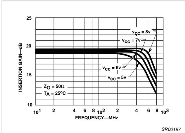
Figure 5. Insertion Gain vs Frequency ( $S_{21}$ )
