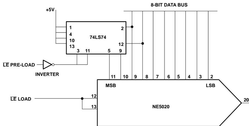
Figure 12. Pre-loading the 2 MSBs to Provide a Single-Step Output
