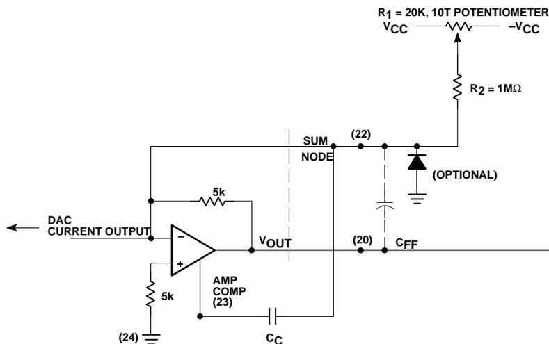
Figure 14. Zero-Scale Adjustment
