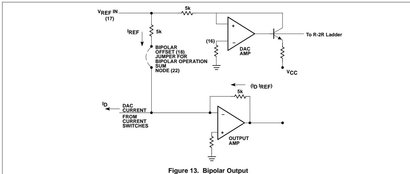
Figure 13. Bipolar Output
