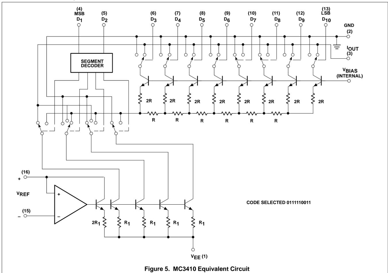
Figure 5. MC3410 Equivalent Circuit
