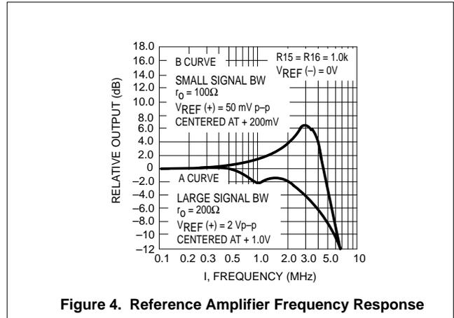
Figure 4. Reference Amplifier Frequency Response
