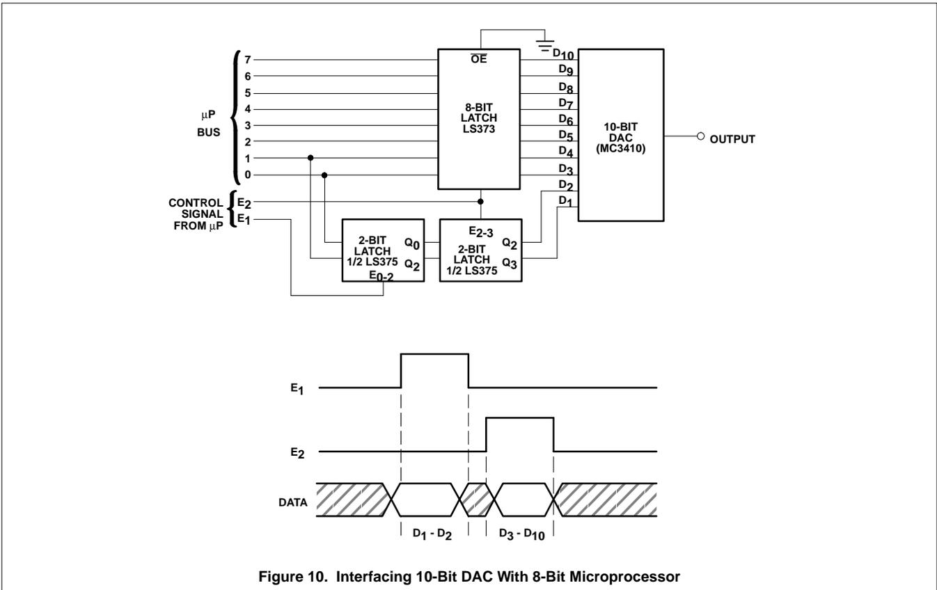
Figure 10. Interfacing 10-Bit DAC With 8-Bit Microprocessor
