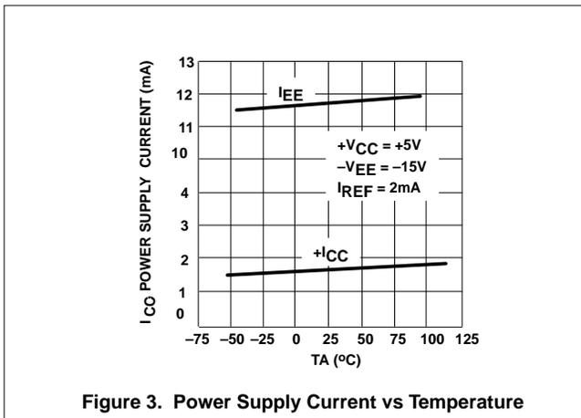
Figure 3. Power Supply Current vs Temperature
