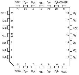
\* All V<sub>CC</sub> and V<sub>CCO</sub> pins are tied together on the die.
