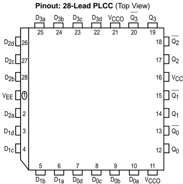
\* All VCC and VCCO pins are tied together on the die.
