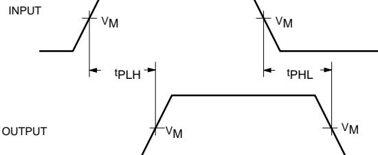
Waveform 1. Input to Output Propagation Delays
