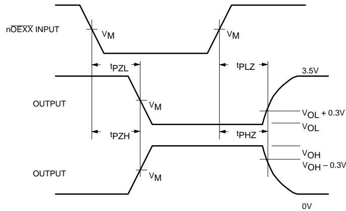
Waveform 2. 3-State Output Enable and Disable Times
