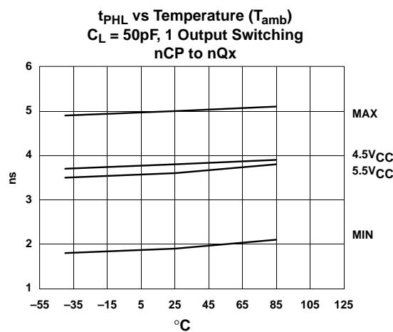
**Adjustment of  $t_{PHL}$  for Load Capacitance and # of Outputs Switching**
