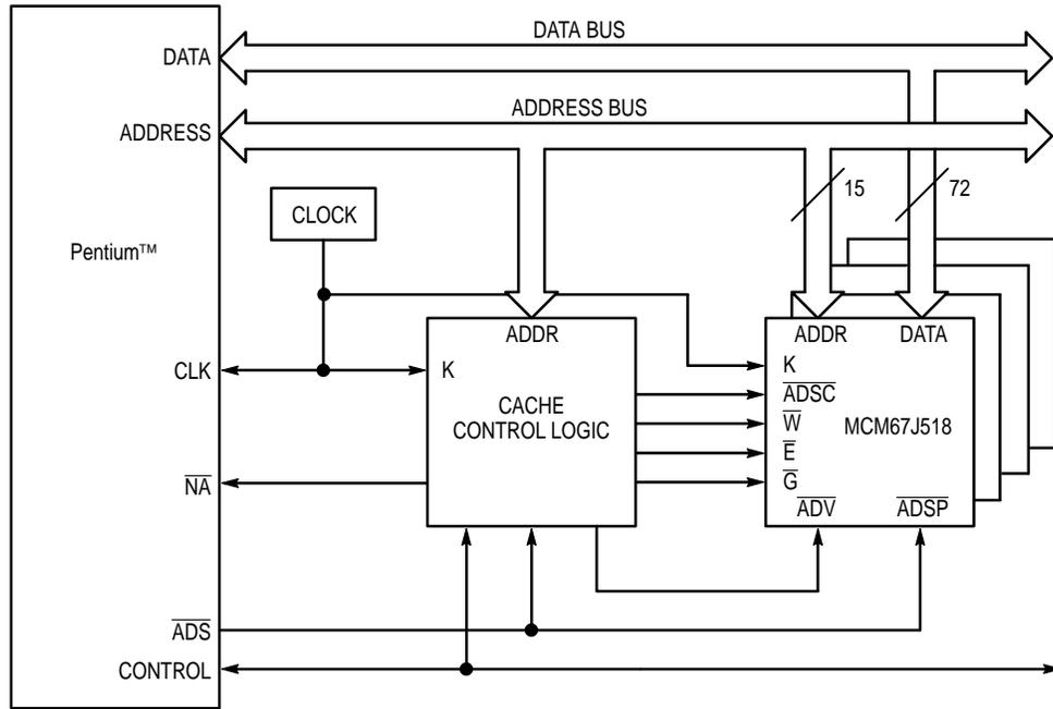
256K Byte Burstable, Secondary Cache Using
