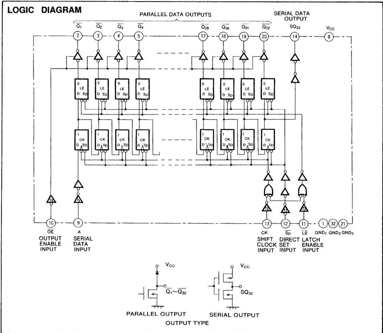
32-BIT LED DRIVER WITH SHIFT REGISTER AND LATCH
