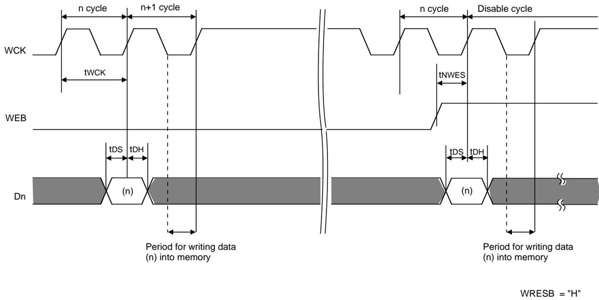
Input data of n cycle is read at the rising edge after WCK of n cycle and writing operation starts in the WCK low-level period of n+1 cycle. The writing operation is complete at the falling edge after n+1 cycle.
