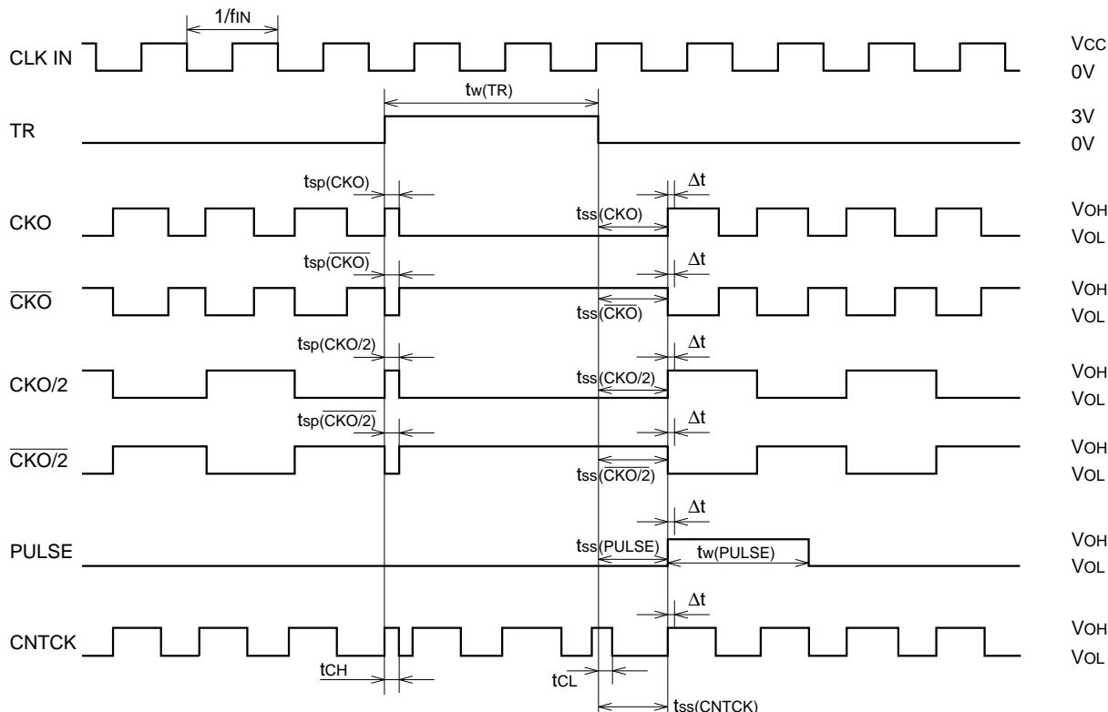
Note 1: tss (CKO,  $\overline{\text{CKO}}$ ,  $\text{CKO}/2$ ,  $\overline{\text{CKO}}/2$  and PULSE) equals the sum of input clock "L" width and  $\alpha$ . Value  $\alpha$  refers to internal delay in M66236. Under environment where temperature and Vcc do not change, value  $\alpha$  and tss are kept constant. Dispersion of tss under such conditions is defined as  $\Delta t$  [synchronizing precision (jitter)].
