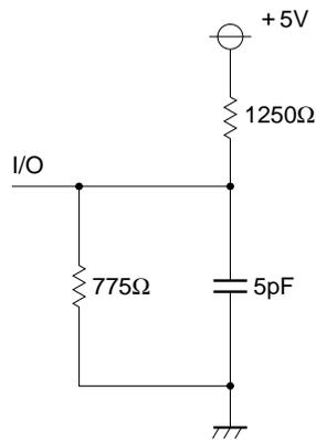
**Fig 2. I/O Output Load
