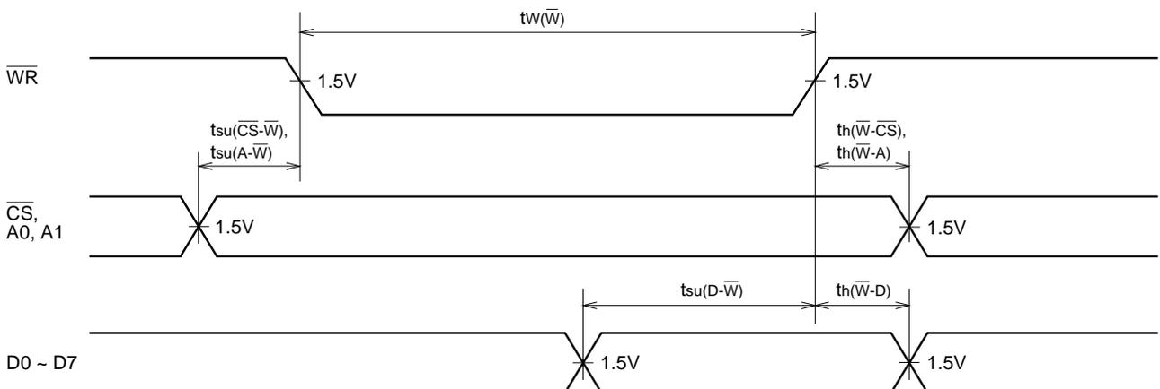
**Write operation internal processing time**
