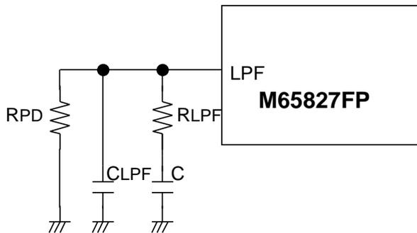
Since the adjustment - free VCO is built in, the adjustment - free PLL circuit can be formed by connecting a resistor and capacitors to the LPF(Low Pass Filter) pin.
