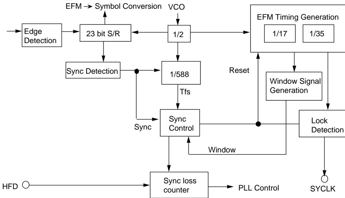
**Fig. 4: Frame synchronize control part block diagram**
