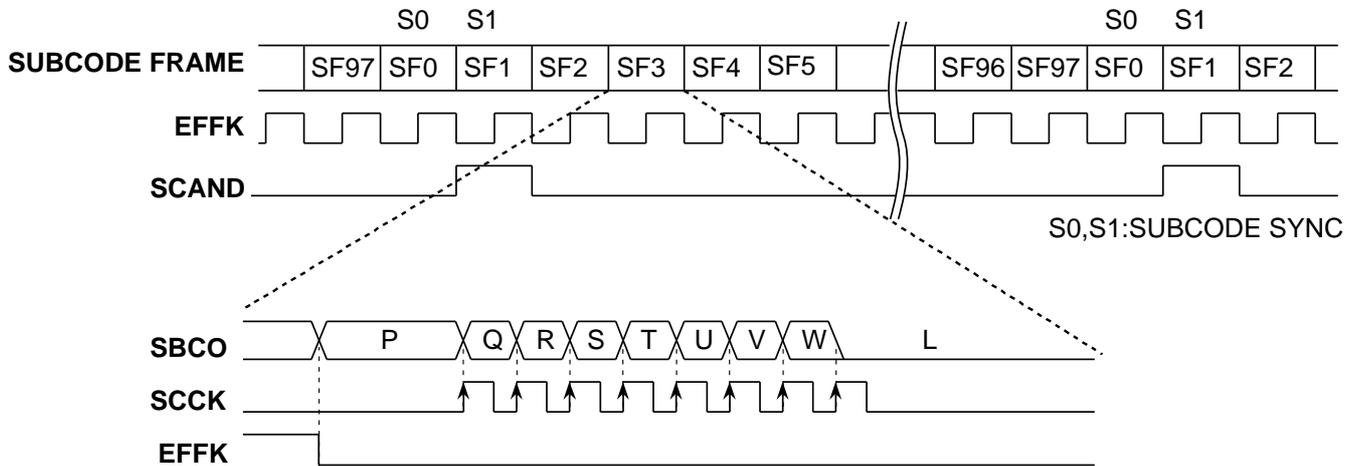
Subcode data synchronization status SCAND outputs "H" only when subcode synchronization patterns both S0 and S1 (S0 AND S1) are detected within a both fixed area of internal synchronization protection circuit.
