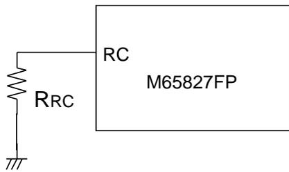
The frequency gain of the VCO of the EFM-PLL can be controlled by connecting the external resistor between RC pin and GND.
