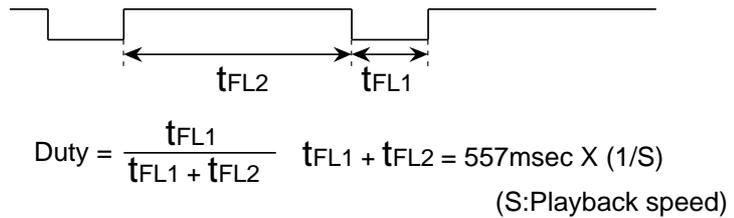
When mute data continue for a long time, PLL sometimes become hard to lock up. When the FLPDIS register at address 01h is "L", false-lock protection circuit adds stimulation to VCO control terminal which causes the PLL to lock up. False-lock protection circuit operates while false-lock protection clock is "L" ( $t_{FL1}$ ) to increase VCO oscillation frequency.
