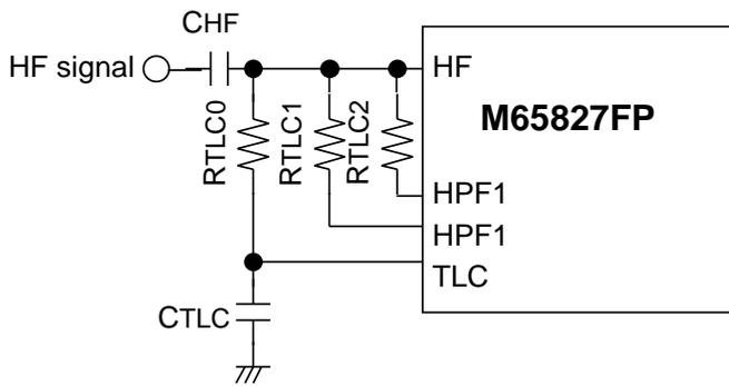
The slice level control circuit is formed by connecting resistors and capacitors to the HF(High - frequency signal input) and TLC (Slice level control output) pins.
