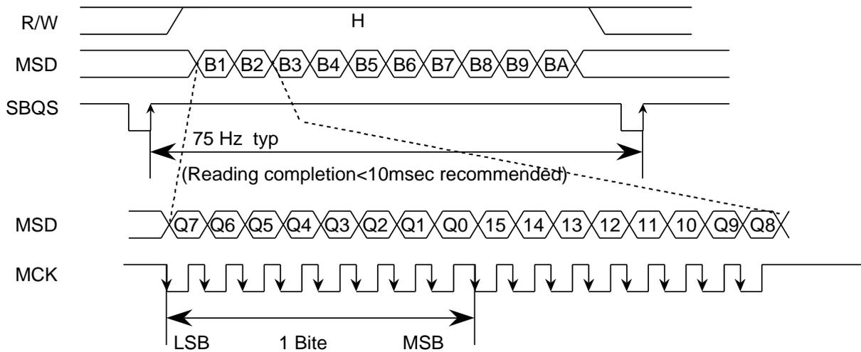
Subcode Q data which is stored in internal 80 bit register can be read in serial clock of MCU. When R / W signal is "H", MSD are settled to output. By inputting 80 ck to MCK pin between two rising edges of SBQS pin, MSD pin output subcode Q data at the falling edge of MCK. Subcode Q data are output reversed MSB, LSB in 8 bit unit. SBQS pin output "L", when next condition are satisfied and internal register can be read.
