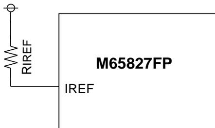
Resistors must be connected between the IREF pin and VDD in order to set the reference current used in determining the current values of the TLC pin and LPF pin, the comparator operating current of the slice level control circuit, and VCO free - run frequency.
