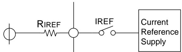
IREF=L: The analog block change to sleep mode by stopping the reference current to analog circuit.
