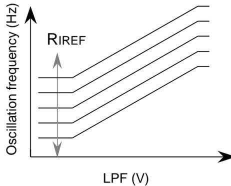
The gain of the oscillation frequency (  $f / V$  ) can be controlled by the external resistor RRC and the minimum oscillation frequency can be controlled by the external resistor RREF. And the frequency divider ratio of the internal VCO of the EFM-PLL can be also controlled by the address 05h resistor for each playback speed.
