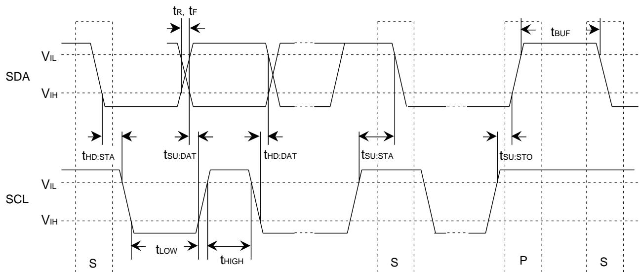
**8-BIT 8CH I<sup>2</sup>C-BUS D-A CONVERTER WITH BUFFER AMPLIFIERS****I<sup>2</sup>C BUS FORMAT**
