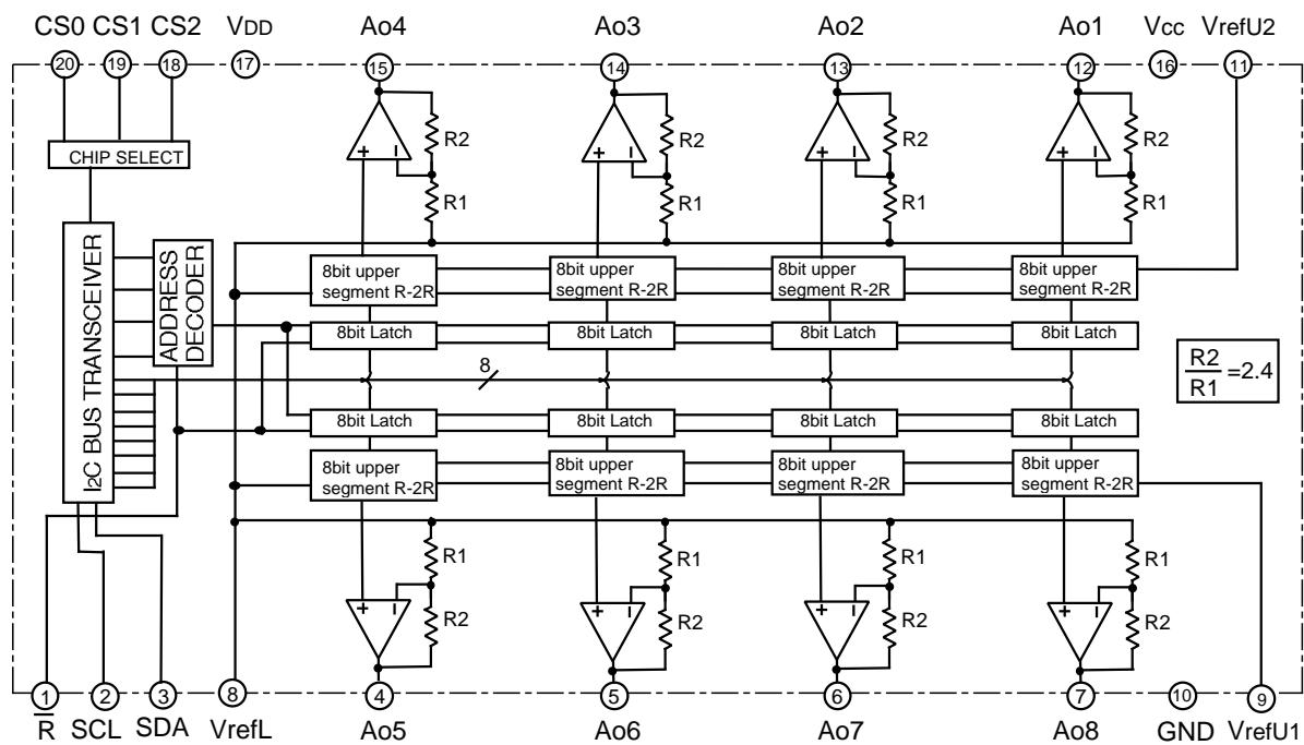
**8-BIT 8CH I<sup>2</sup>C-BUS D-A CONVERTER WITH BUFFER AMPLIFIERS****EXPLANATION OF TERMINALS**
