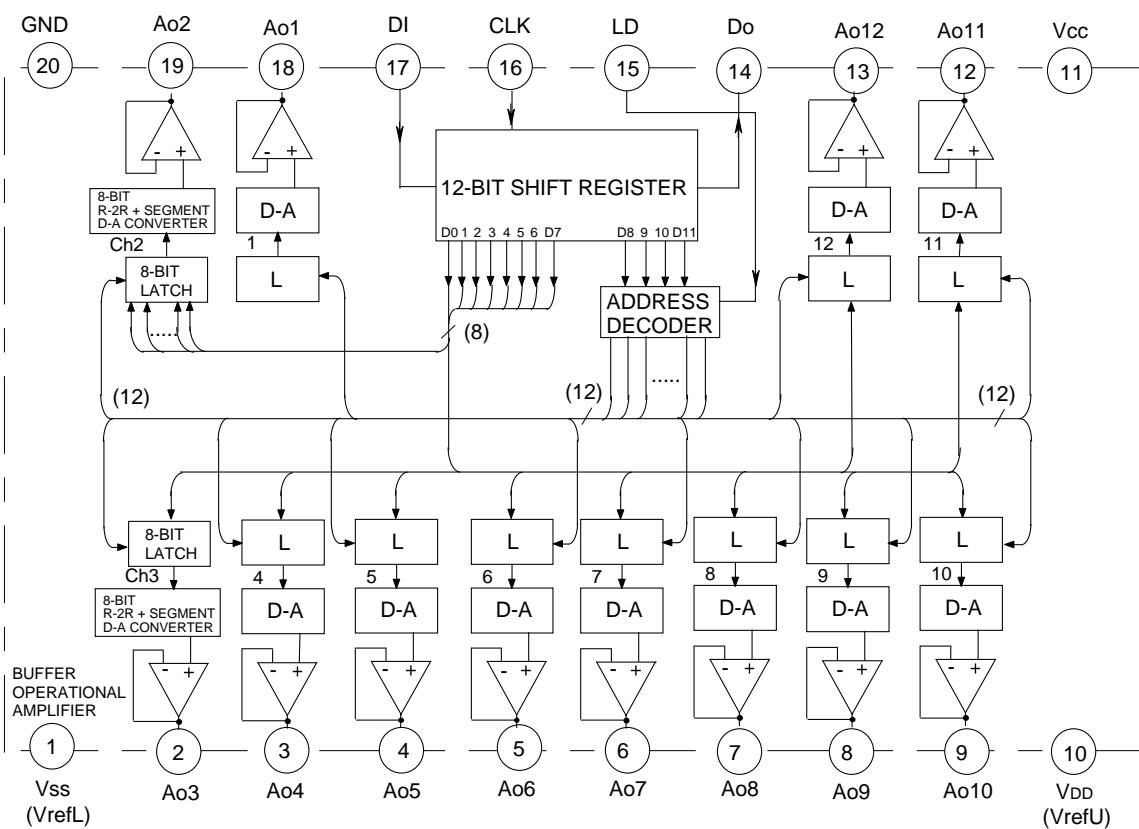
**3V TYPE 8-BIT 12CH D-A CONVERTER WITH BUFFER AMPLIFIERS****EXPLANATION OF TERMINALS**
