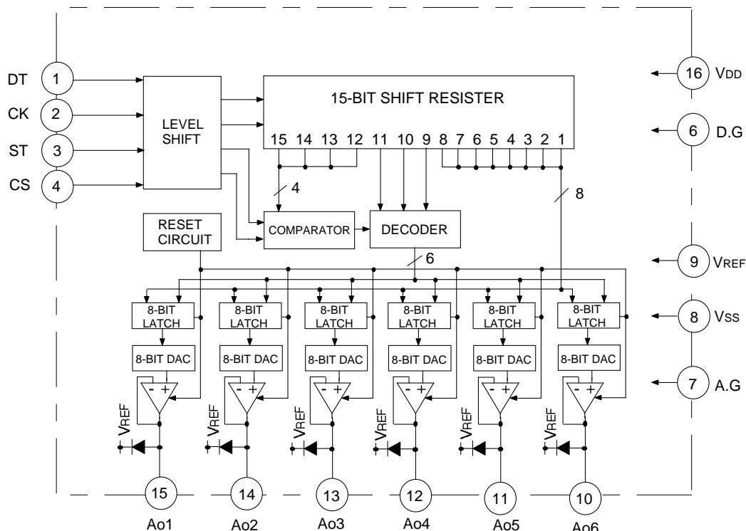
**8-BIT 6CH D-A CONVERTER WITH BUFFER AMPLIFIERS****EXPLANATION OF TERMINALS**
