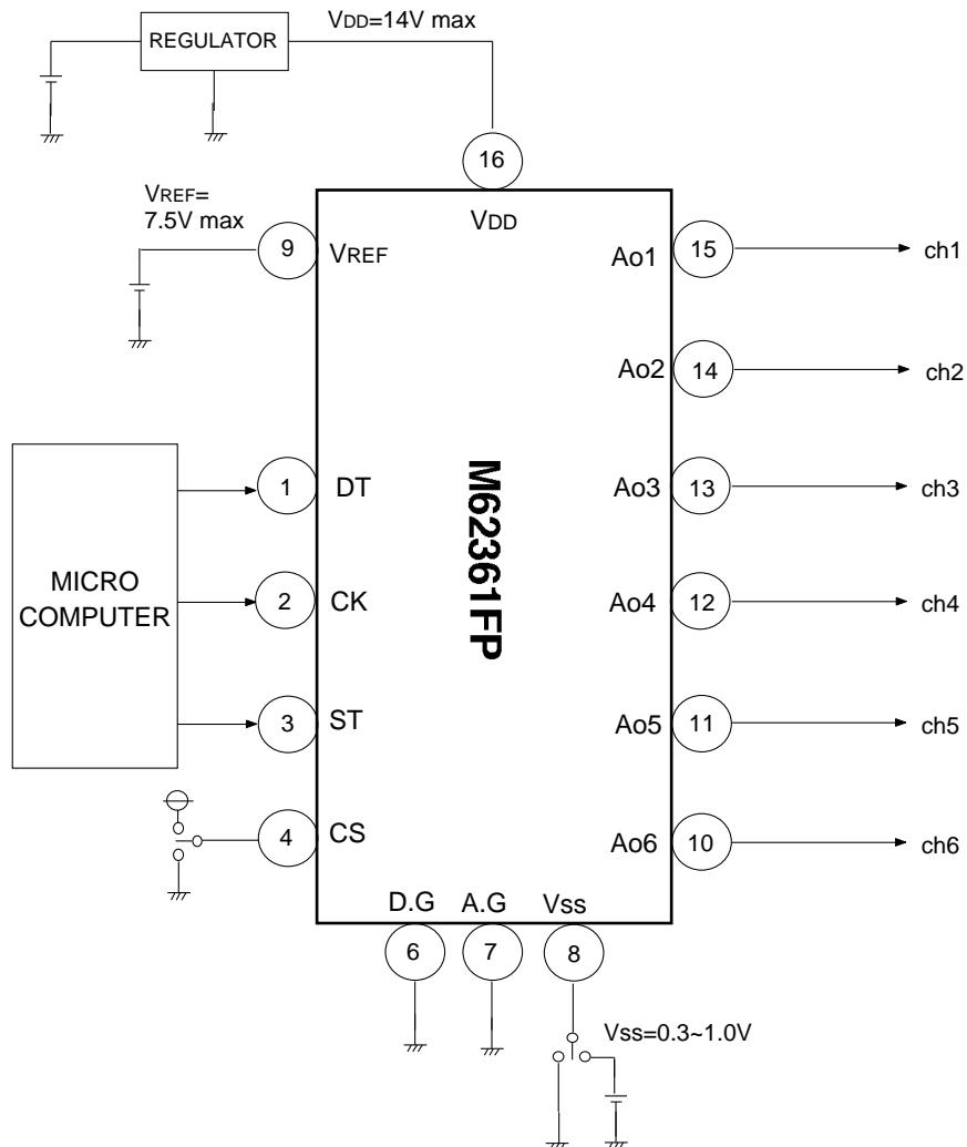
When ⑧ pin is GND, Ao output is  $0.3 \sim V_{REF} - 1 \text{ LSB}$
