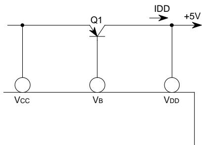
Since it capable of driving external PNP Tr. base up to 20mA, it can supply current of
