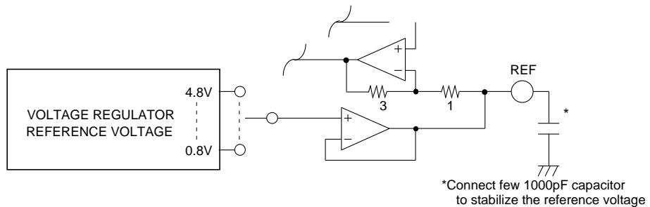
Select the desire reference voltage to be detected by serial data from the microcomputer.
