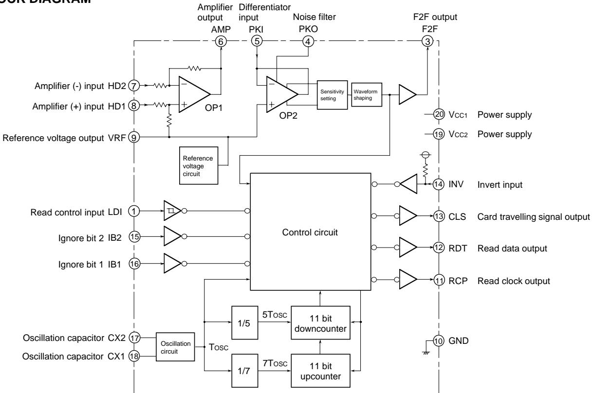
**F2F MAGNETIC STRIPE ENCODING CARD READER****I/O CIRCUIT**
