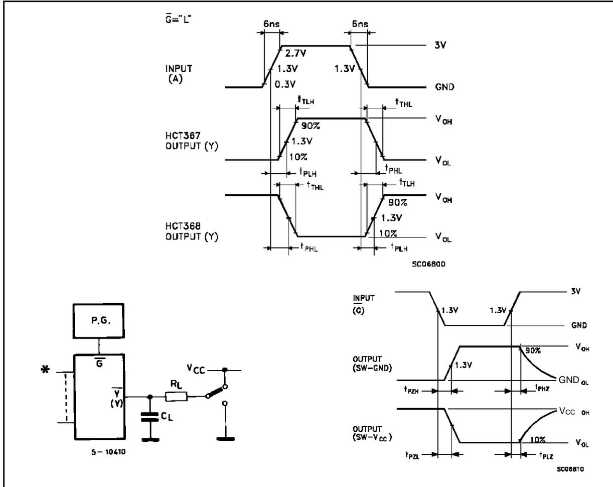
Note : Such a logic level shall be applied to each input that the output voltage stays in the apposite side to the switch connection level, when the output is enabled.
