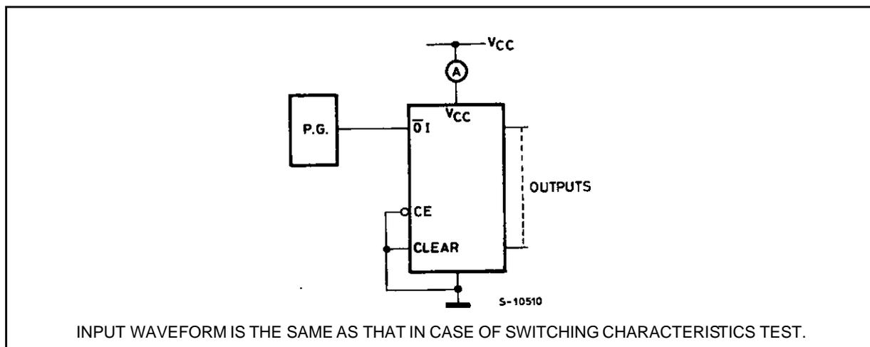
INPUT WAVEFORM IS THE SAME AS THAT IN CASE OF SWITCHING CHARACTERISTICS TEST.
