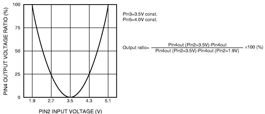
**V PARA AMP GAIN CONTROL VOLTAGE VS. OUTPUT AMPLITUDE**
