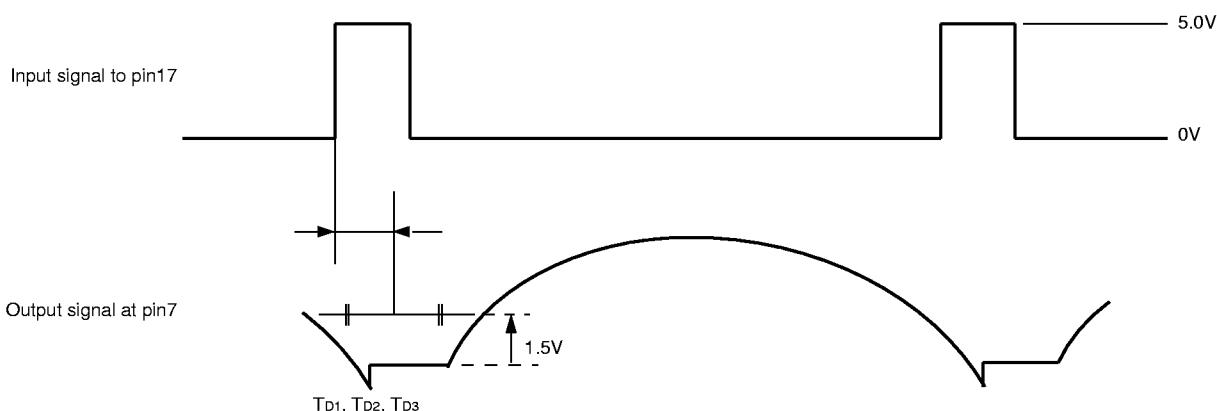
**D<sub>d</sub> Delay temperature drift**
