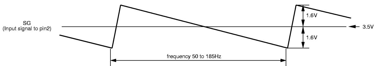
**ELECTRICAL CHARACTERISTICS TEST METHOD****I<sub>CC1</sub> Circuit current1**
