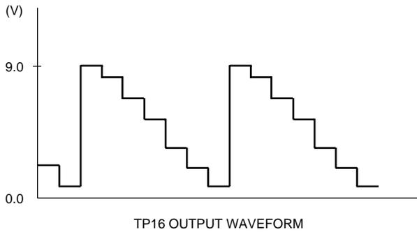
Gradually increase the amplitude of SG8 from 700mV, and measure the amplitude of the TP16 output waveform when the upper side of the waveform becomes distorted.
