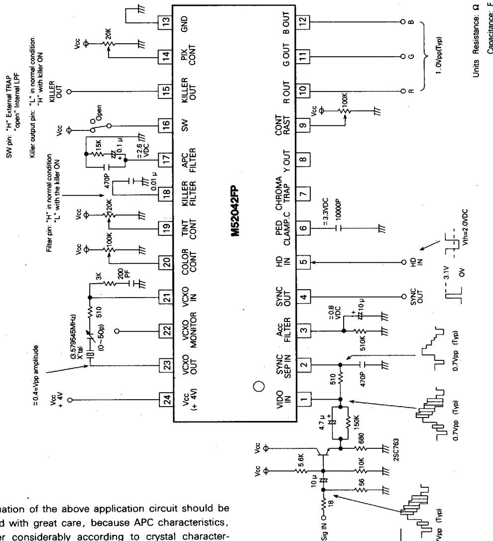
The evaluation of the above application circuit should be performed with great care, because APC characteristics, etc. differ considerably according to crystal characteristics and board pattern.
