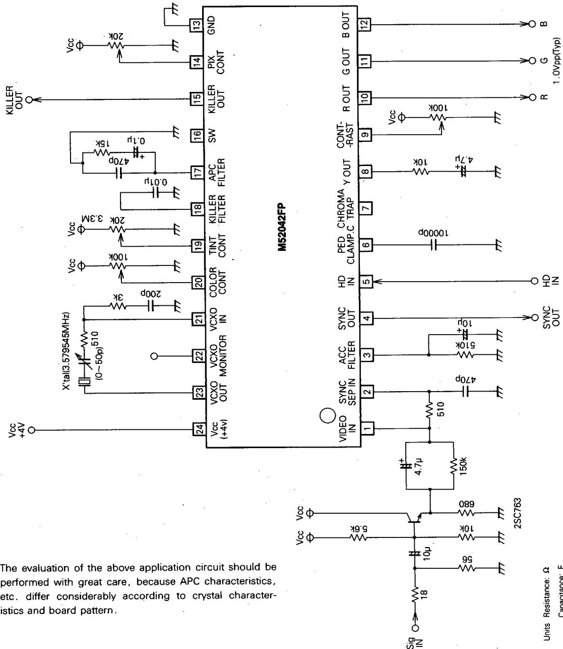
The evaluation of the above application circuit should be performed with great care, because APC characteristics, etc. differ considerably according to crystal characteristics and board pattern.
