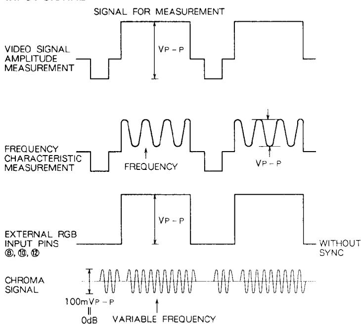
Unless otherwise specified, input a video signal of 1V<sub>P-P</sub> to Pin ⑨ (sync separation input).
