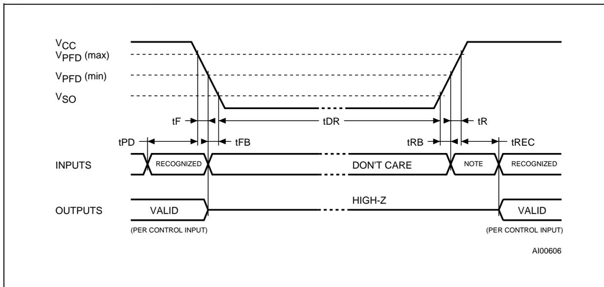
**Note:** Inputs may or may not be recognized at this time. Caution should be taken to keep  $\bar{E}$  high as  $V_{CC}$  rises past  $V_{PFD}(\text{min})$ . Some systems may perform inadvertent write cycles after  $V_{CC}$  rises above  $V_{PFD}(\text{min})$  but before normal system operations begin. Even though a power on reset is being applied to the processor, a reset condition may not occur until after the system clock is running.
