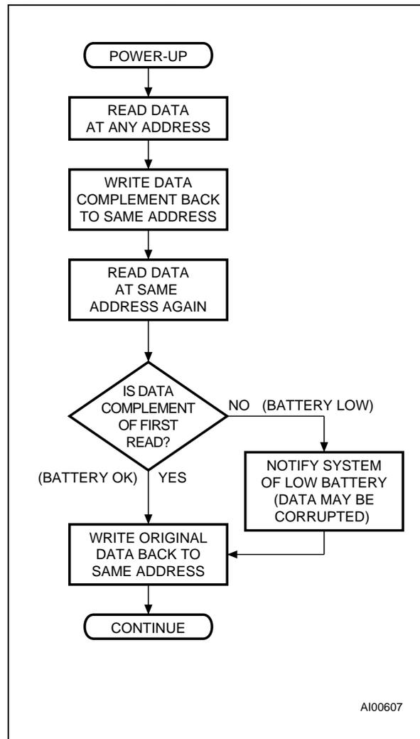
Figure 10. Supply Voltage Protection
