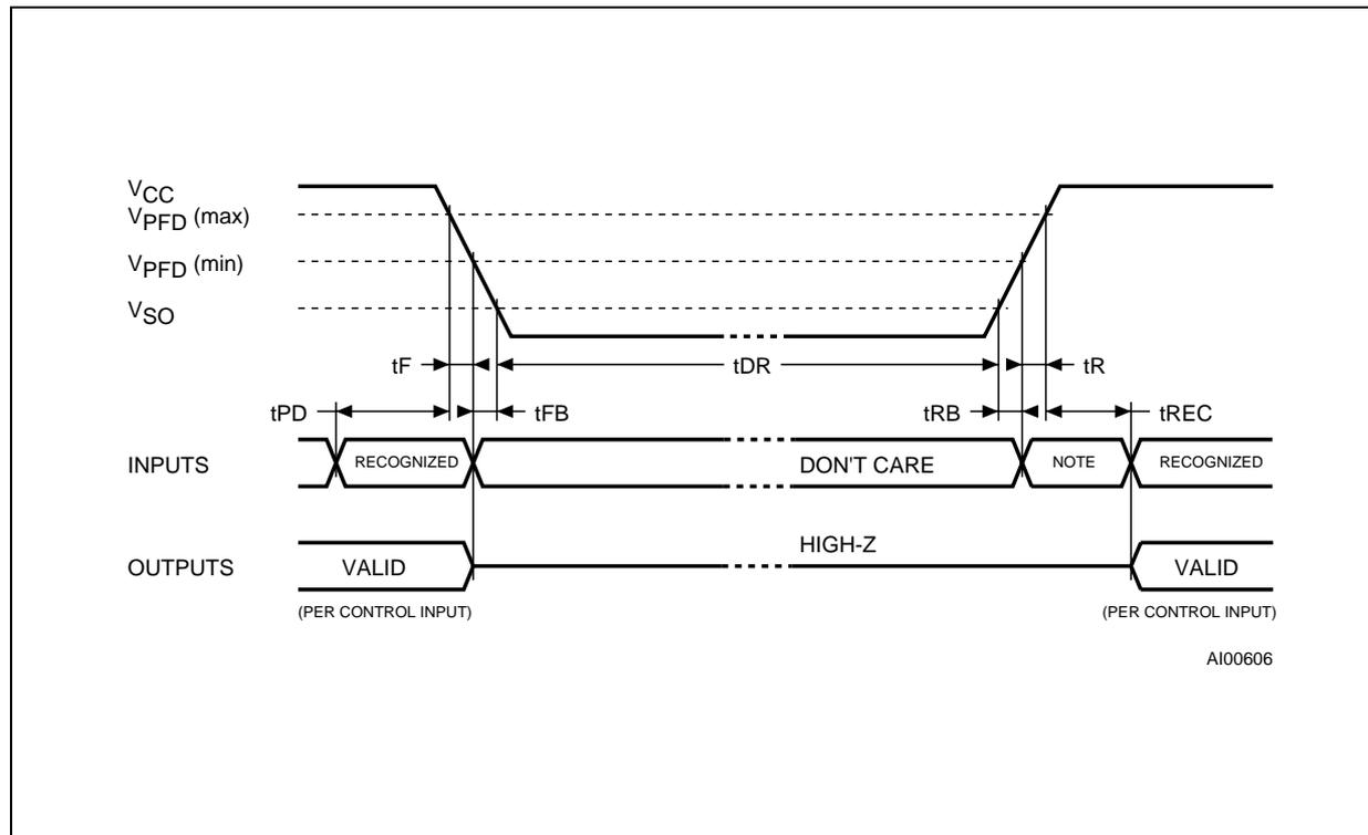
**Note:** Inputs may or may not be recognized at this time. Caution should be taken to keep  $\bar{E}$  high as  $V_{CC}$  rises past  $V_{PFD}(\text{min})$ . Some systems may perform inadvertent write cycles after  $V_{CC}$  rises above  $V_{PFD}(\text{min})$  but before normal system operations begin. Even though a power on reset is being applied to the processor, a reset condition may not occur until after the system clock is running.
