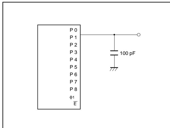
Fig. 58 Testing circuit for ports P0-P8,  $\phi$ 1
