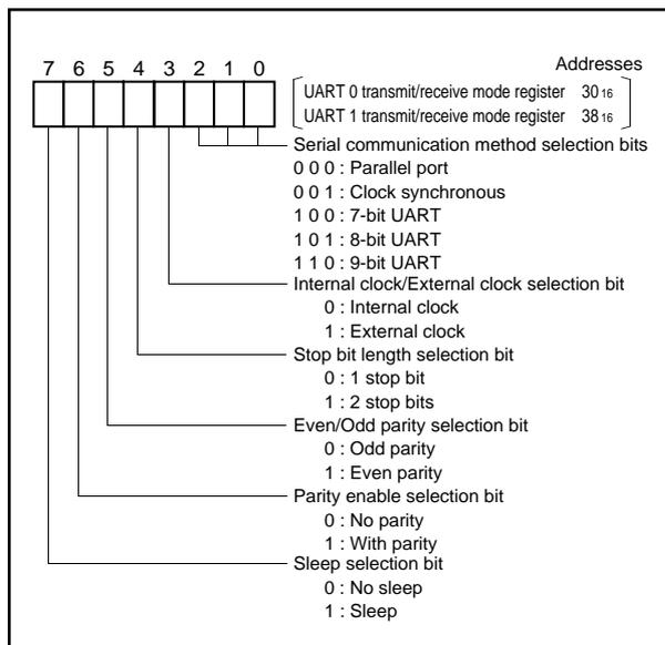
Fig. 34 UART <sub>i</sub> Transmit/Receive mode register bit configuration
