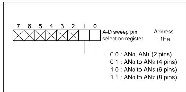
Fig. 45 A-D sweep pin selection register configuration
