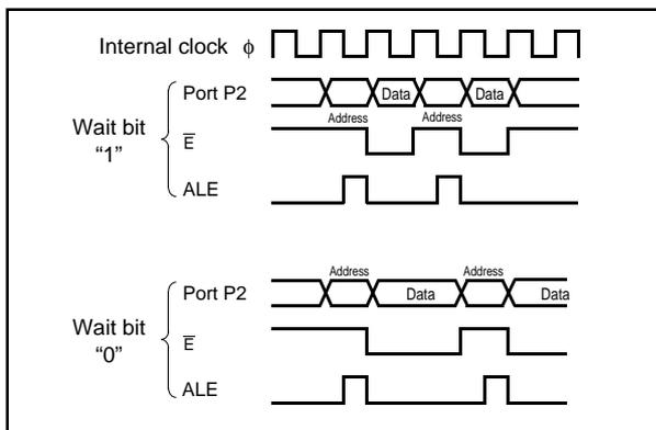
**Fig. 54 Relationship between wait bit and access time**
