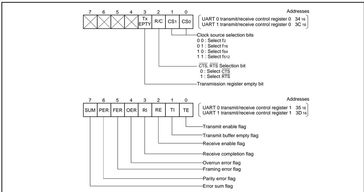
Fig. 37 UARTi Transmit/Receive control register bit configuration
