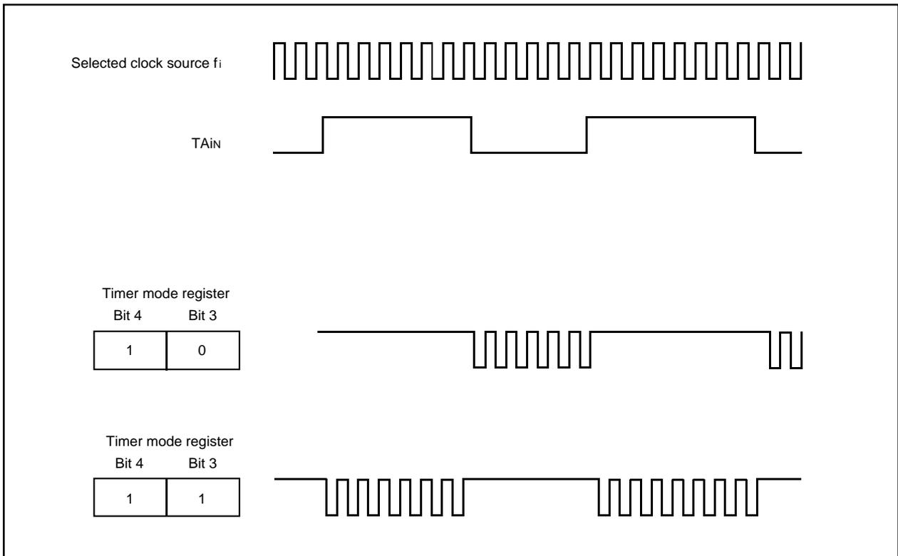
**Fig. 14** Count waveform when gate function is available
