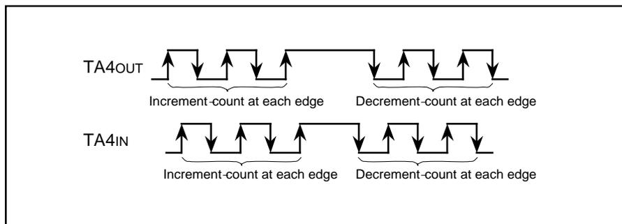
**Fig. 18 Two-phase pulse processing operation of timer A4**
