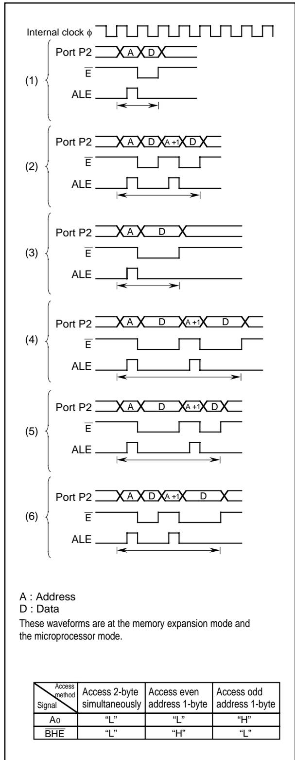
**Fig. 5 Relationship between access method and signals A<sub>0</sub> and BHE**
