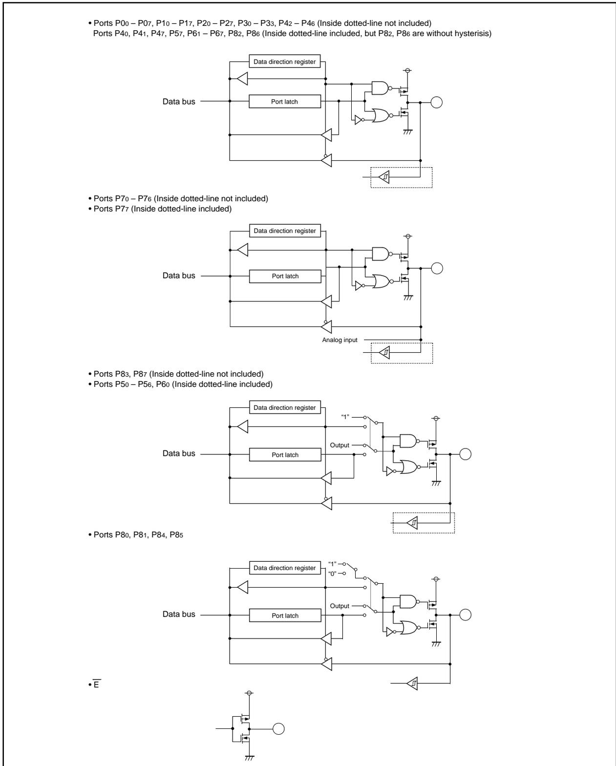
Fig. 50 Block diagram for ports P8 to P0 in single-chip mode and the  $\bar{E}$  pin output
