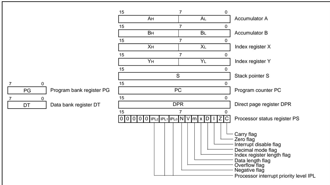
Fig. 3 Register structure
