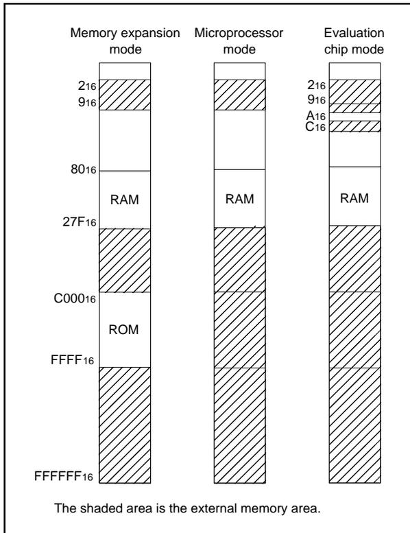
**Fig. 53 External memory area for each processor mode**
